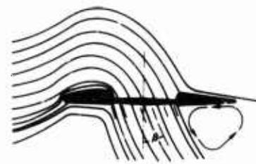
Fig. 35 Cross section of lift-fan flow field.
