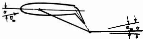
Fig. 10 Side View of Non-Planar Trailing Vortex System Used in Davenport Methodology.
