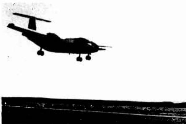
Fig. 3 Photograph of Augmented Jet-STOL Research Aircraft.
