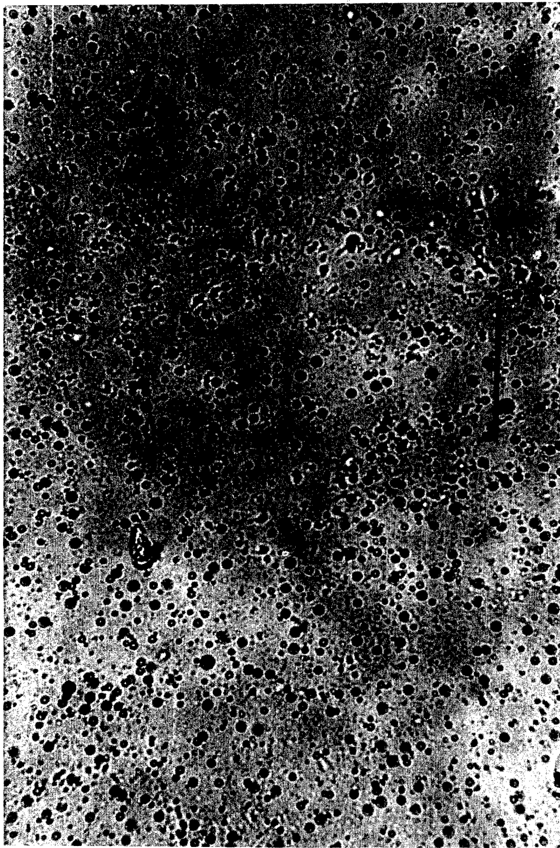
Figure 27. Optical photomicrograph of the same emulsion of Component II curing agent prepared using the Manton-Gaulin Homogenizer, after standing for 30 days.
