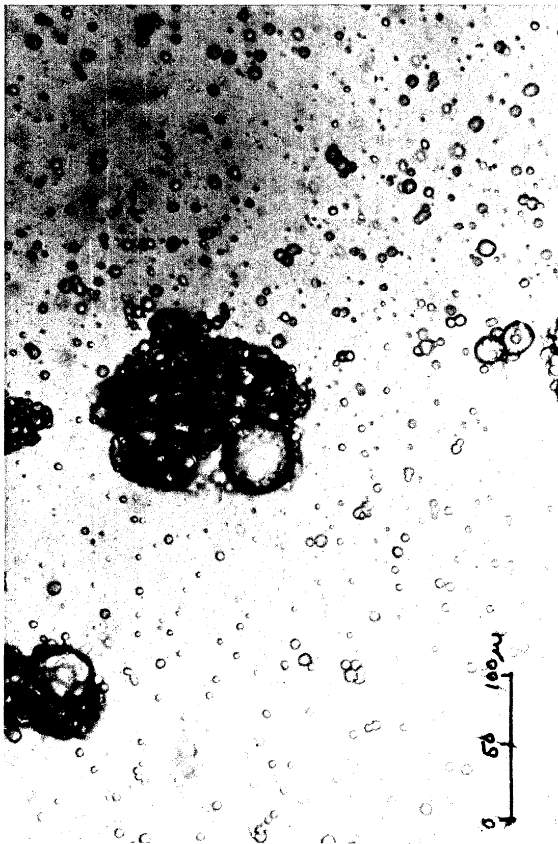
Figure 23. Optical photomicrograph of an emulsion of 70:30 Versamid 115-xylene mixture prepared with simple stirring, after standing for 2 hours.
