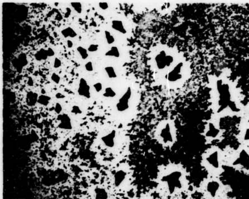
Fig. 28. \text{As}_2\text{S}_3 deposit on uncoated (left) and pre-coated KCl substrate (50x).
