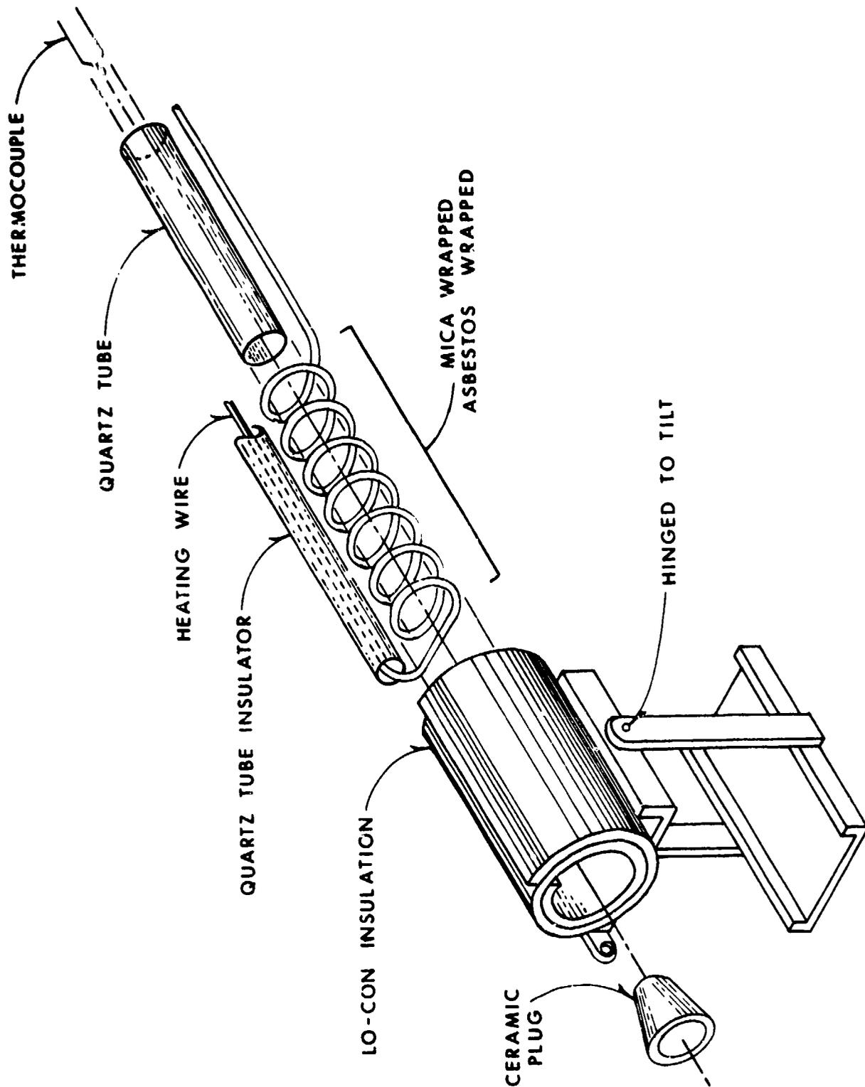
Figure 3. High Temperature Furnace
