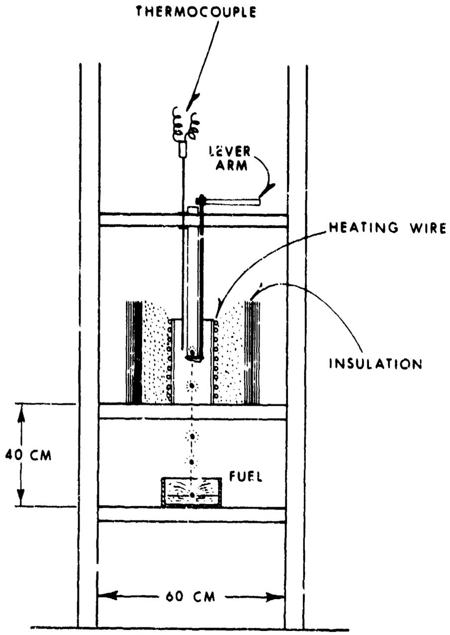
Figure 1. Ignition Apparatus
