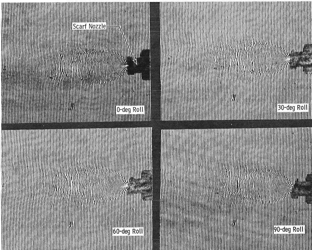
Figure 4. Holographic finite fringe interferogram of scarf nozzle plume.
