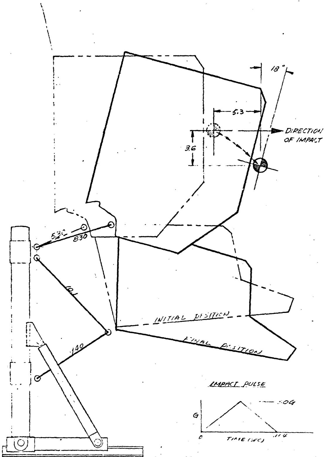
Figure 12. Seat Displacement in Horizontal Impact - 95th Percentile.
