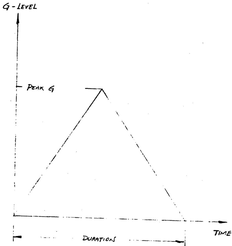
Figure 6. Typical Impact Pulse
