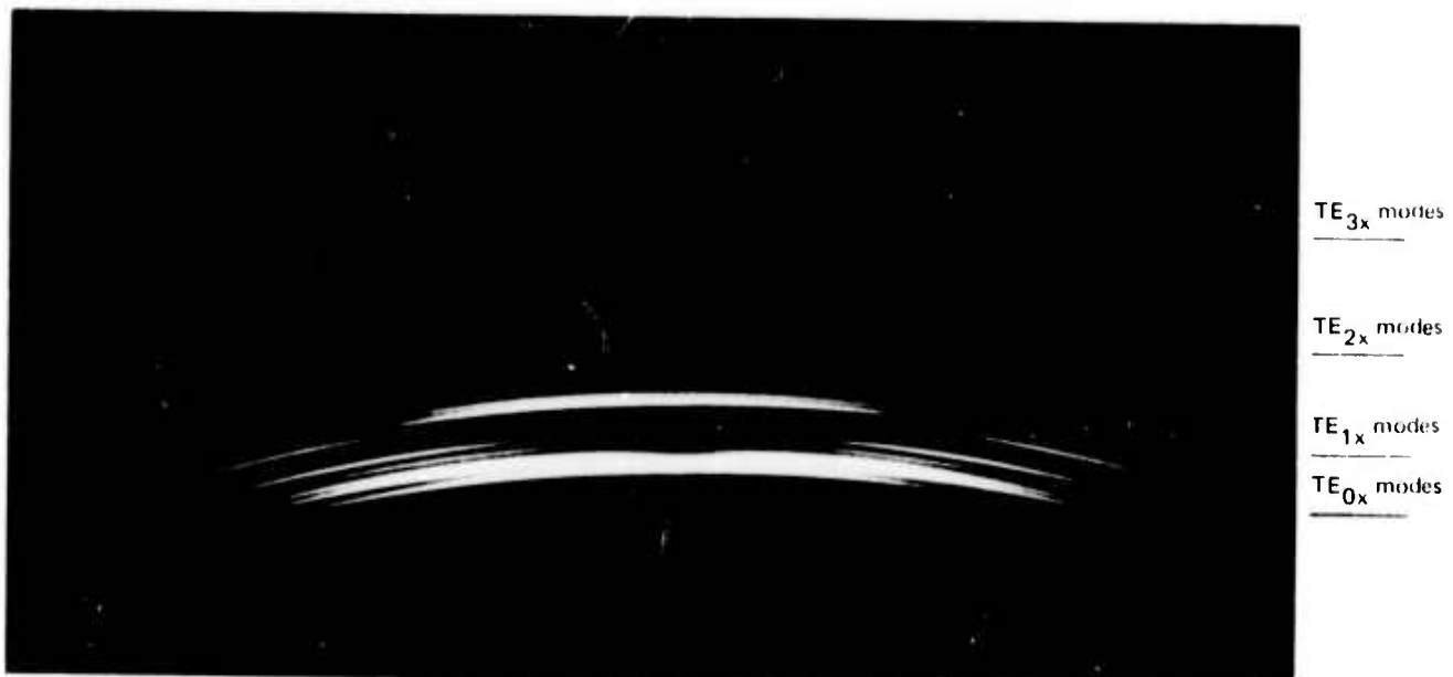
Figure 41. The spectrum of mode lines from a prism coupler on a 7-by-2- \mu\text{m} guide. The lowest line in each band corresponds to the fundamental transverse mode; higher lines correspond to higher-order modes.
