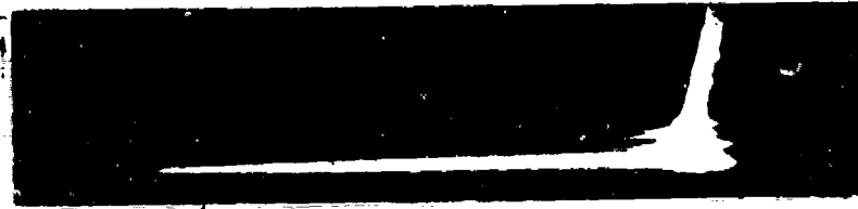
Figure 82. Photography of the transition of combustion of a mixture of 10% PS+90% AP to detonation ( r=15 \mu\text{m} , \rho=0.65 \text{ g/cm}^3 , p=1 \text{ atm} open tube with a length of 100 cm). [PS = PS, polystyrene; \text{KXA} = AP, ammonium perchlorate]
