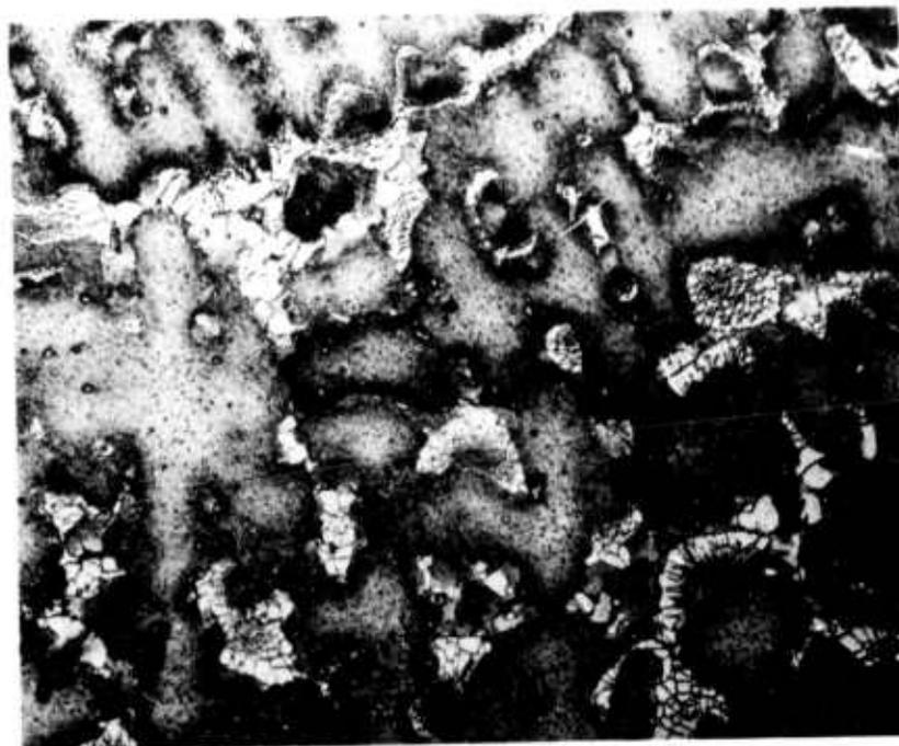
Figure 20. TRW VI A casting same as Fig. 19. Center of web section. Same features as thick section except coarser microstructure. Porosity associated with  $\gamma - \gamma'$  eutectic in lower right. Marble's reagent. 250X
