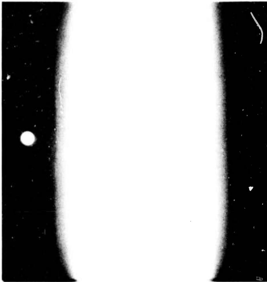
Figure 15. X-ray photograph of IN-738 casting made as in Fig. 13. 1470°C pouring temperature, 400°C mold temperature. Hole in center left is thermocouple tube. Surface defects visible as small circles. No porosity evident.
