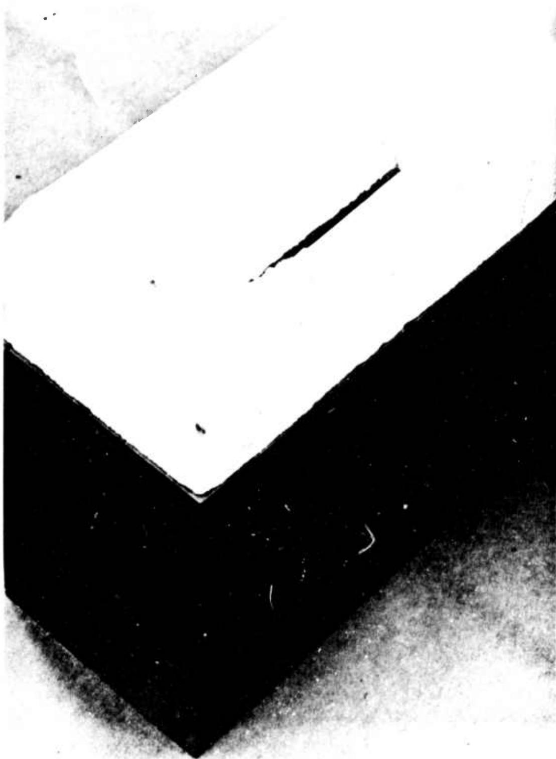
Figure 3. Pouring basin. Basin is "vee" shaped with a slit opening in bottom, the width of the mold cavity. It is made of high fired zircon.
