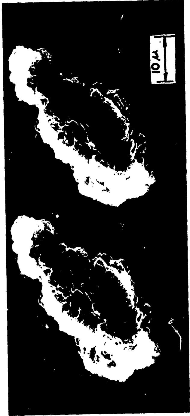
Figure 3.24 A typical large wear particle from the gear lubricating oil. Note that the particle looks as if a large number of thin sheets are pressed together.
