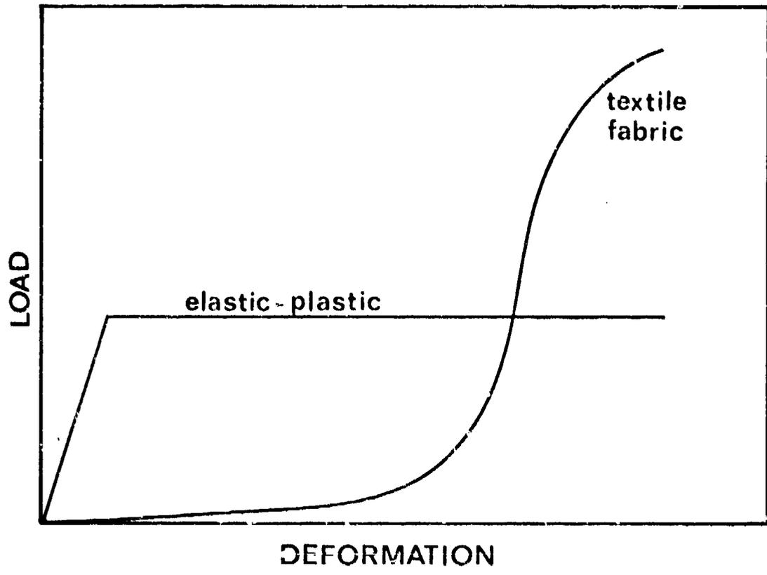
FIG.1 Different shapes of load-deformation curves
