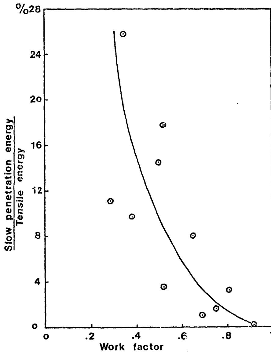
FIG.23 Effect of work factor on energy absorption
