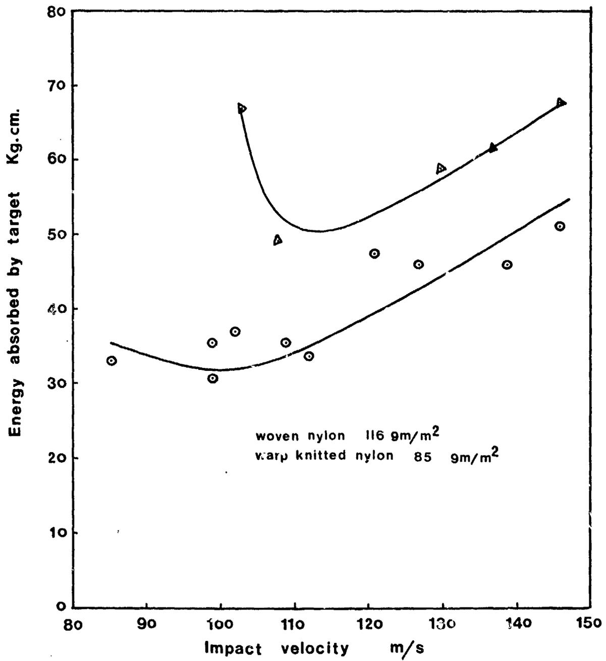
FIG.11 Effect of initial velocity on energy absorption
