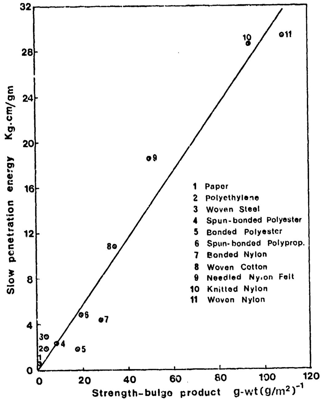
FIG.22 Relation between strength-bulge product and energy in slow penetration
