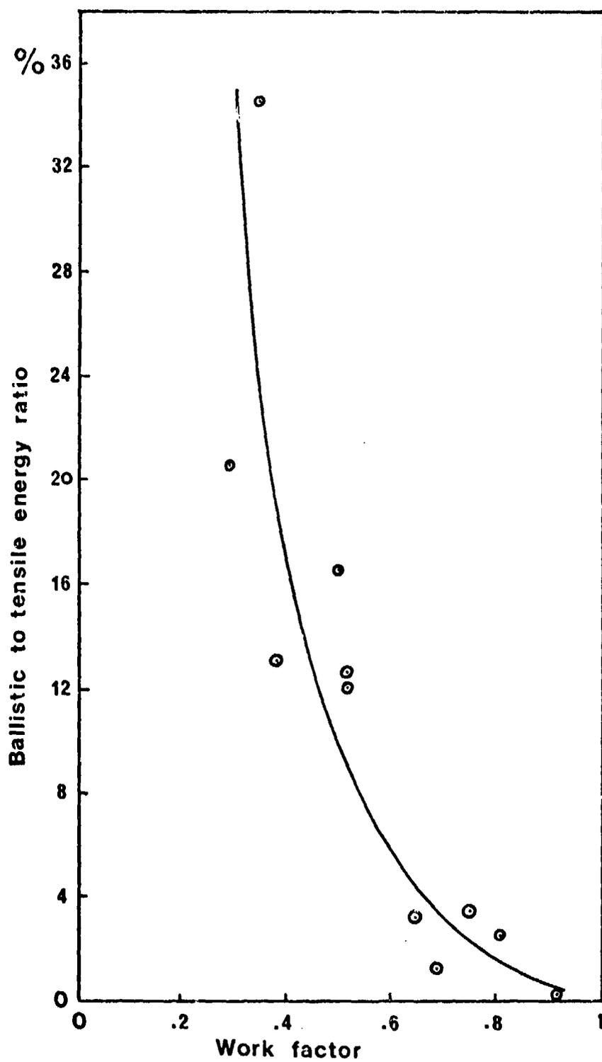
FIG.24 Effect of work factor on energy absorption
