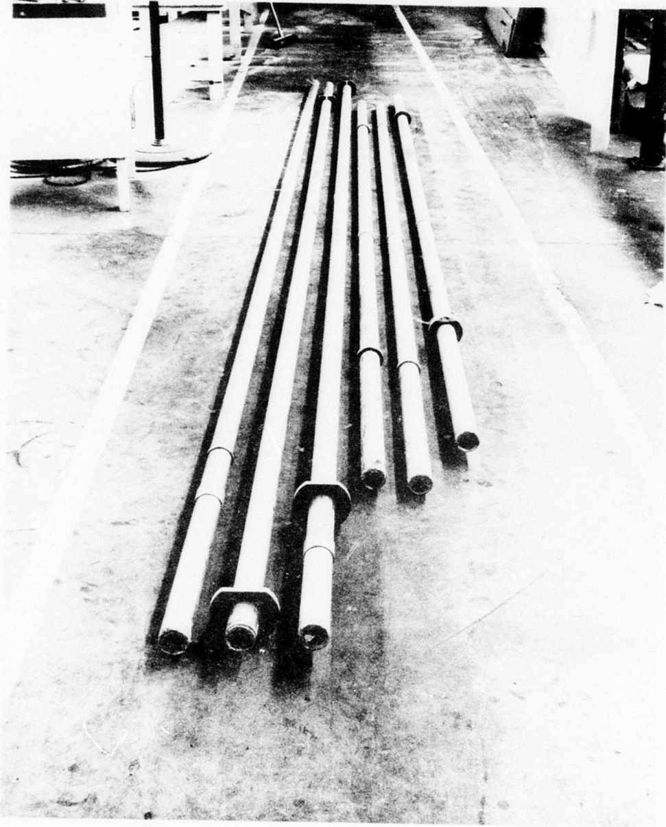
Figure 25. Tube winding hardware ready to have plastic bags attached.
