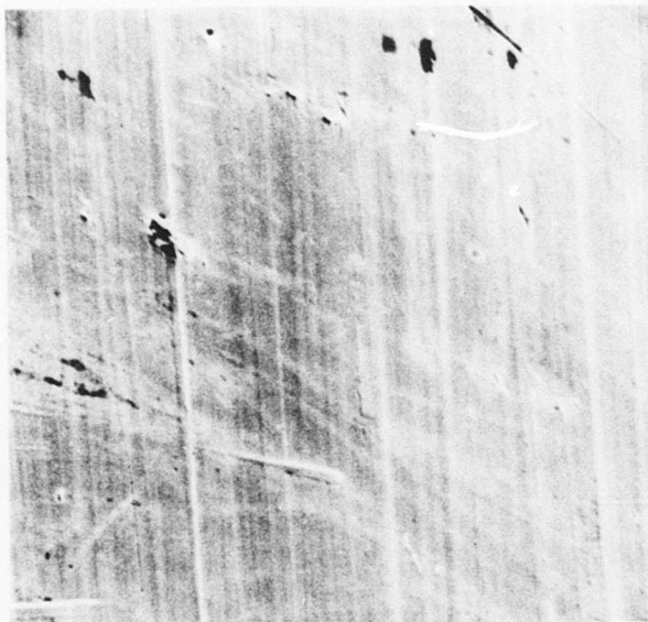
1000X Typical noncontact surface, showing finishing marks
