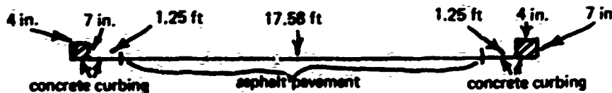
Fig. C-1. Roadway cross section.
