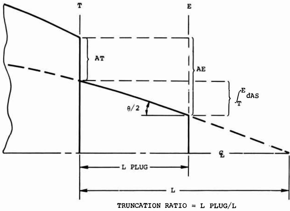
Figure 671. Identification of Typical Plug Nozzle Parameters.
