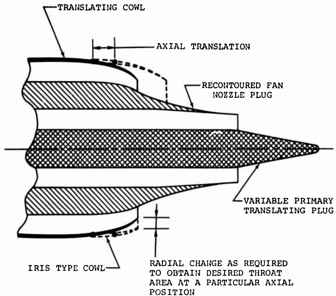
Figure 679. Nozzle Configuration for Improving Variable-Fan Nozzle Performance.
