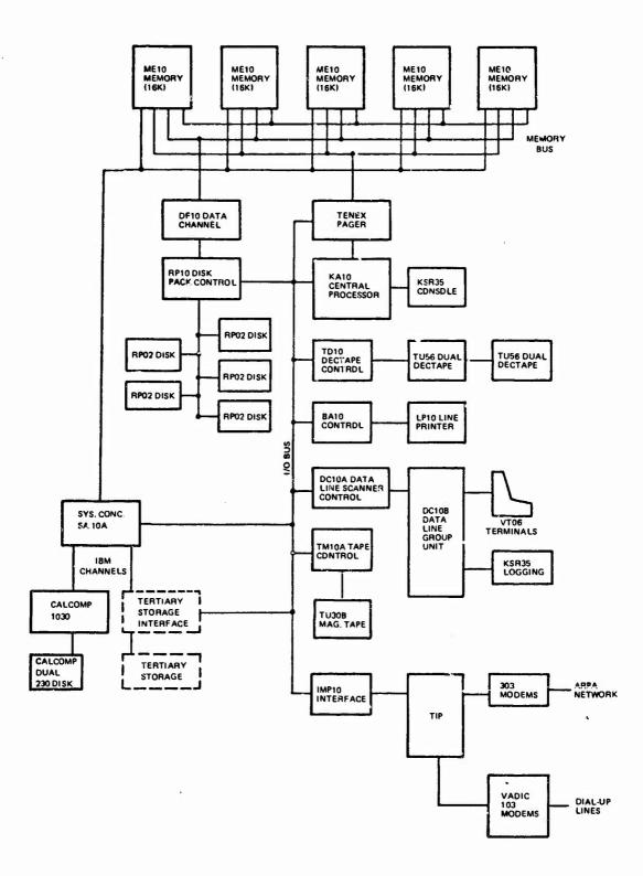
Figure 3. Hardware Block Diagram - CCA Installation (Equipment in dashed outline is planned for 1975)
