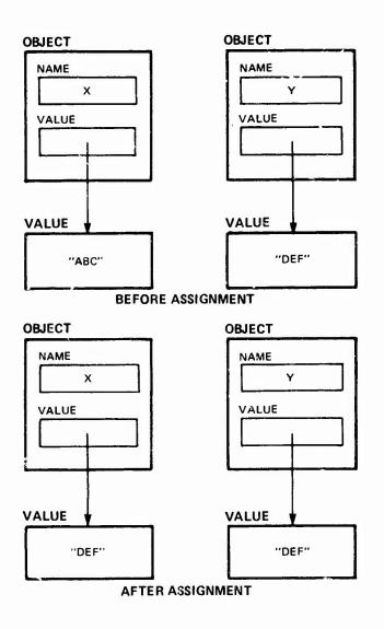
Figure 4-7 Effect of assignment
