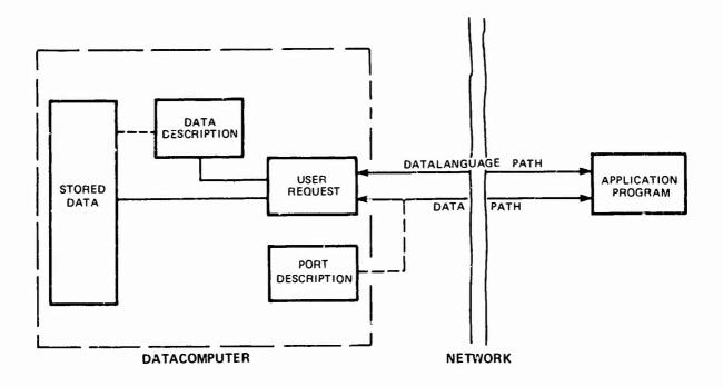
Figure 2-1 A Model of Datacomputer/User Interaction
