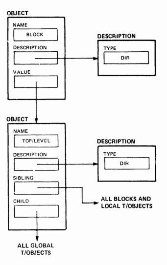
Figure 4-6 BLOCK, TOP/LEVEL and t/objects
