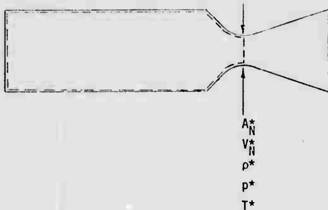
Figure 1a Control Volume for Evaluation of Mass
