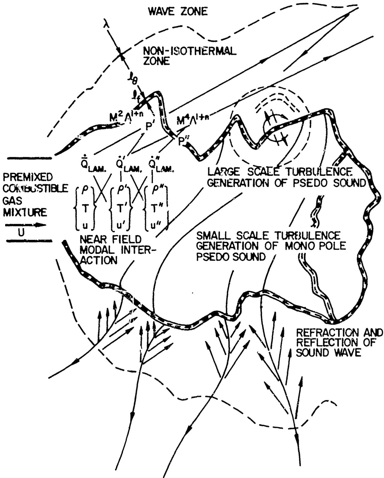
Fig. 2 Schematic diagram of sound generation by a flame: wrinkled laminar flame model.
