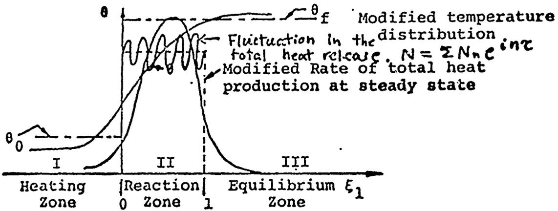
Fig. 6a. Modified Turbulent Steady State Flame Model
