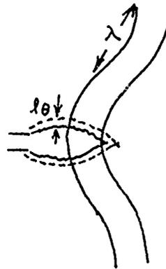
Fig. 3b Refraction and reflection of pressure fluctuation from compact non-isothermal zone  $\lambda \gg l_\theta$ .
