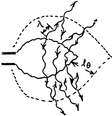
Fig. 3a Refraction and reflection of sound wave in non-isothermal acoustic cavity,  $\lambda \ll l_\theta$ .
