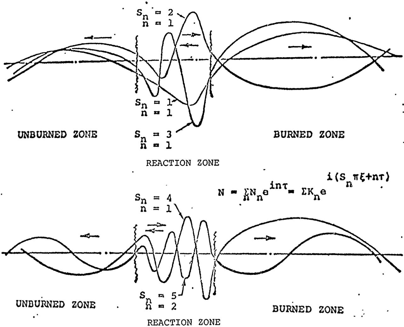
Fig. 6b. Generation and Propagation of Pressure Waves
