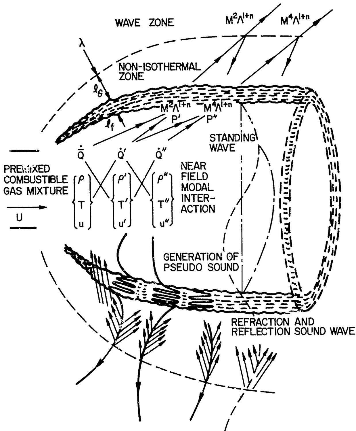
Fig. 1 Schematic diagram of sound generation by a flame: distributed reaction model.
