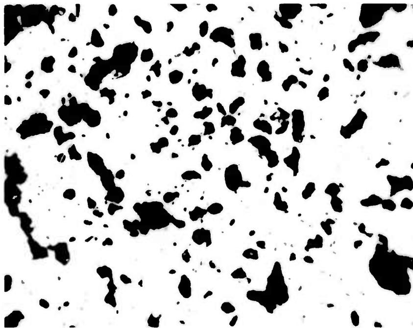
Fig. 19  $B_4C$  sintered with 1%  $Be_2C$  at  $2230^\circ C$  in argon to 85% density. As polished section, 500X.
