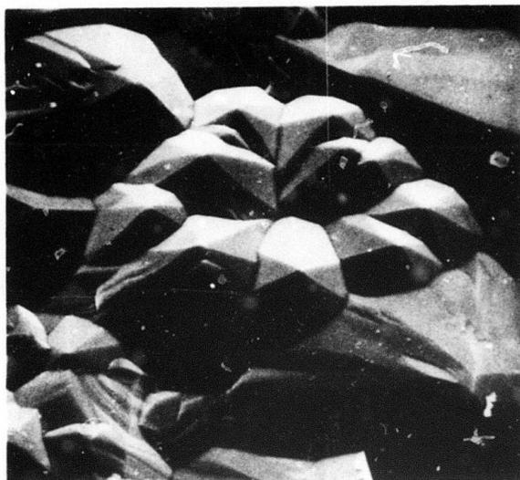
Fig. 2 Scanning electron micrograph of the exposed surface of the CVD Si<sub>3</sub>N<sub>4</sub>. 500X
