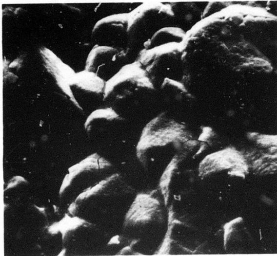
Fig. 4 Scanning electron micrograph of the surface of the CVD Si<sub>3</sub>N<sub>4</sub> after oxidation for 259 hours in air at 1410°C. 500X
