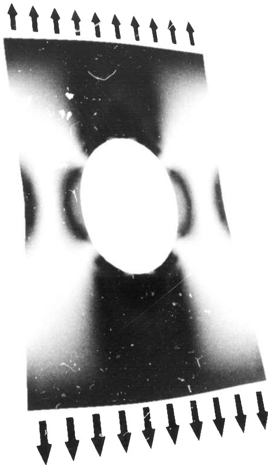
Figure 17. Color stress applied to the display of the results of a finite element analysis of a flat plate with a circular hole.
