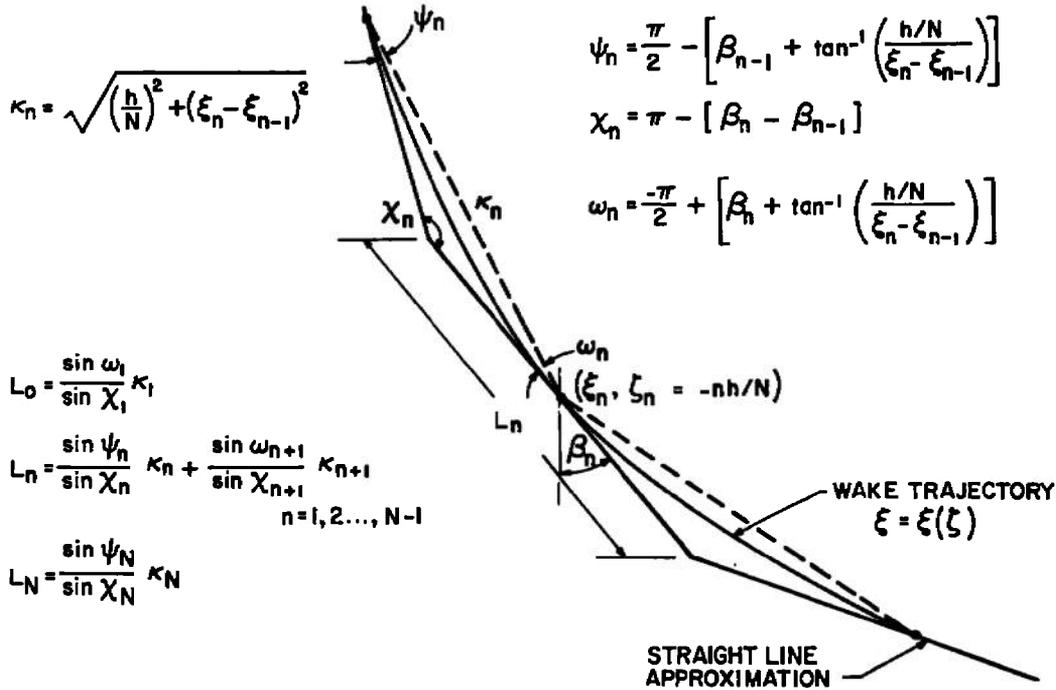
Figure 2. Geometry of straight line approximation to curved jet wake.
