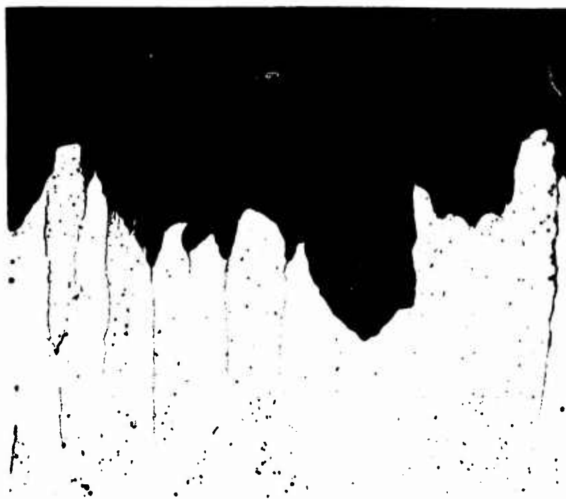
Figure 9. Fiber Oxidation of Specimen Ends, IN-100-Mo (F1) 75X
