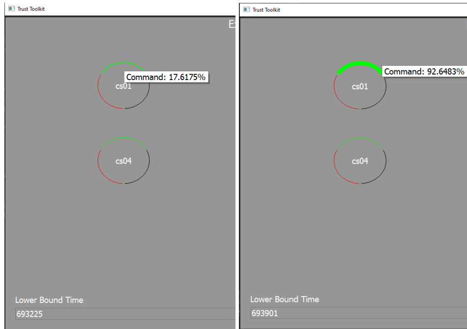
Fig 6 Two visual overviews of communication rates for a selection of crew members. The thickness of a given line indicates the amount of communication on a specific network. Compare the thickness of the top green line (representing communications on the Command network) for cs01 in the left figure with the same line for a different time horizon in the right figure, along with the percentage of communication events represented by each.
