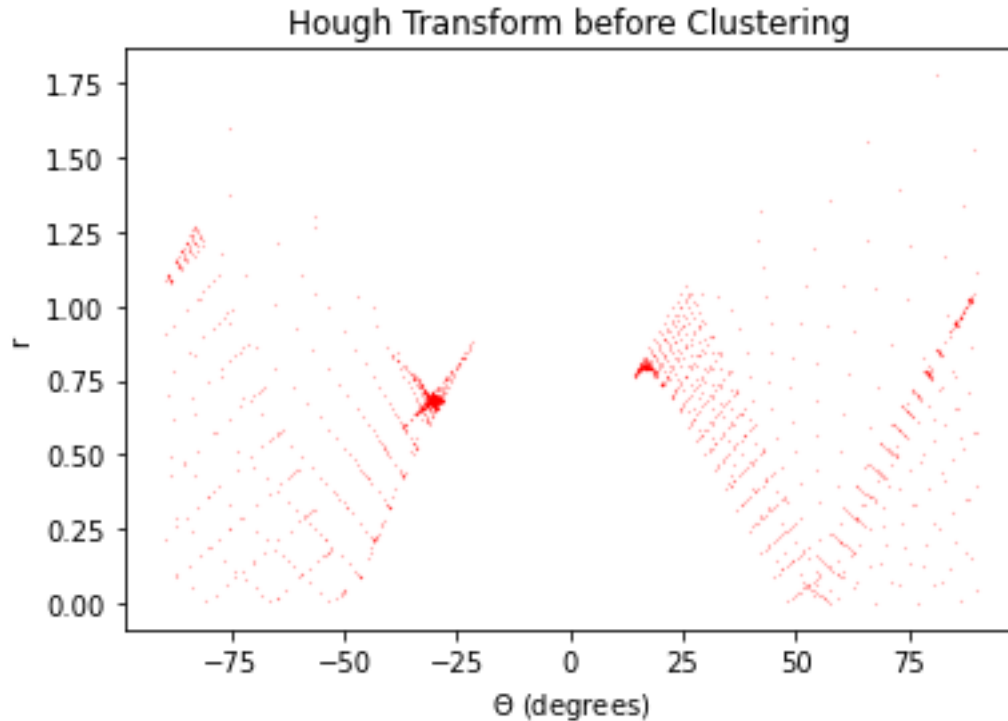
Figure 6. Hough transform as applied to the scaled ship trajectory data.
