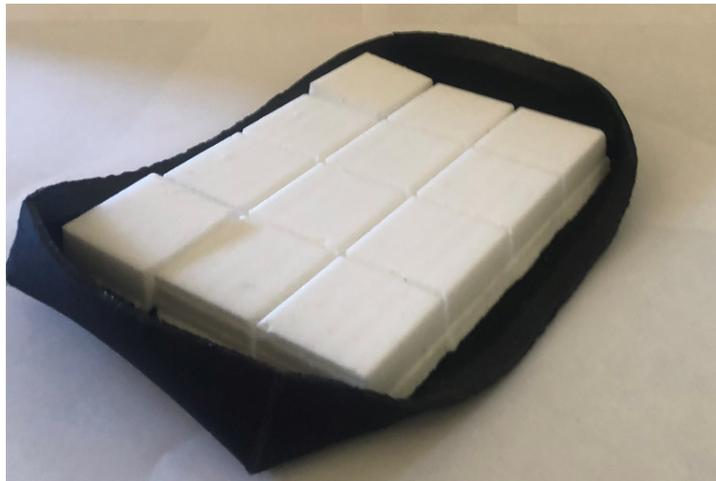
Figure 4.16. Neoprene Pockets Containing Composite
