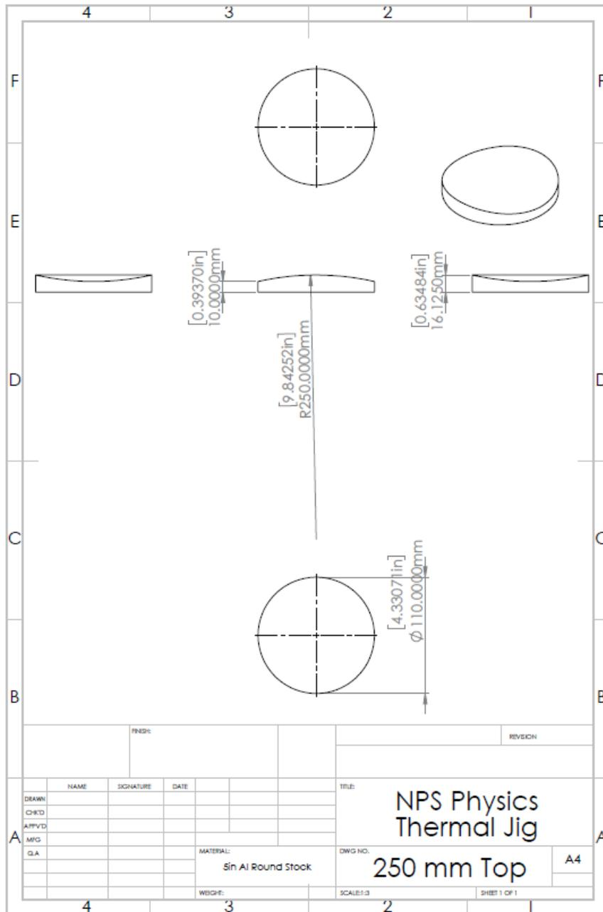
Figure C.4. Jig Top for Composite with  $r=250$  mm
