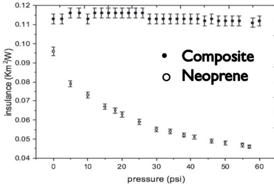
Figure 2.8. Depth Independent Composite Thermal Properties Source: [21]
