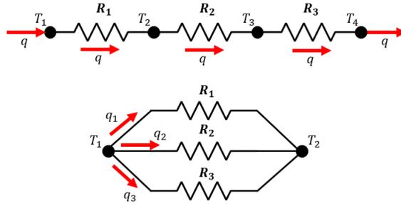
Figure 2.2. A Series Thermal Resistance Network (top) is a linear arrangement of thermal resistors, while a Parallel Thermal Resistance Network (bottom) connects multiple thermal resistors with identical temperature nodes. Source: [17].
