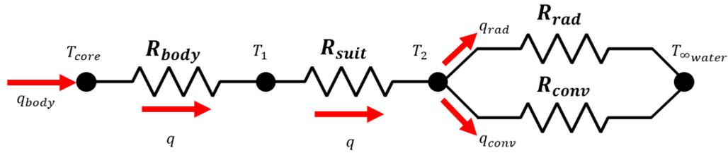
Figure 2.4. Immersed Diver Thermal Circuit with Radiation and Convection
