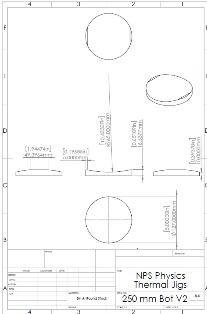
Figure C.3. Jig Bottom for Composite with  $r=250$  mm
