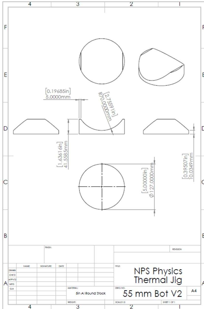
Figure C.1. Jig Bottom for Composite with  $r=50$  mm
