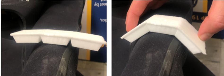
Figure 4.5. Unbent and Bent Composite samples on a dummy wrist
