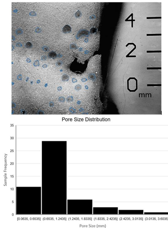
Figure 4.9. High Porosity Image J Tracing and Histogram
