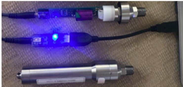
Figure 2.11. Synchronous Data Loggers for Field Testing Source: [18]
