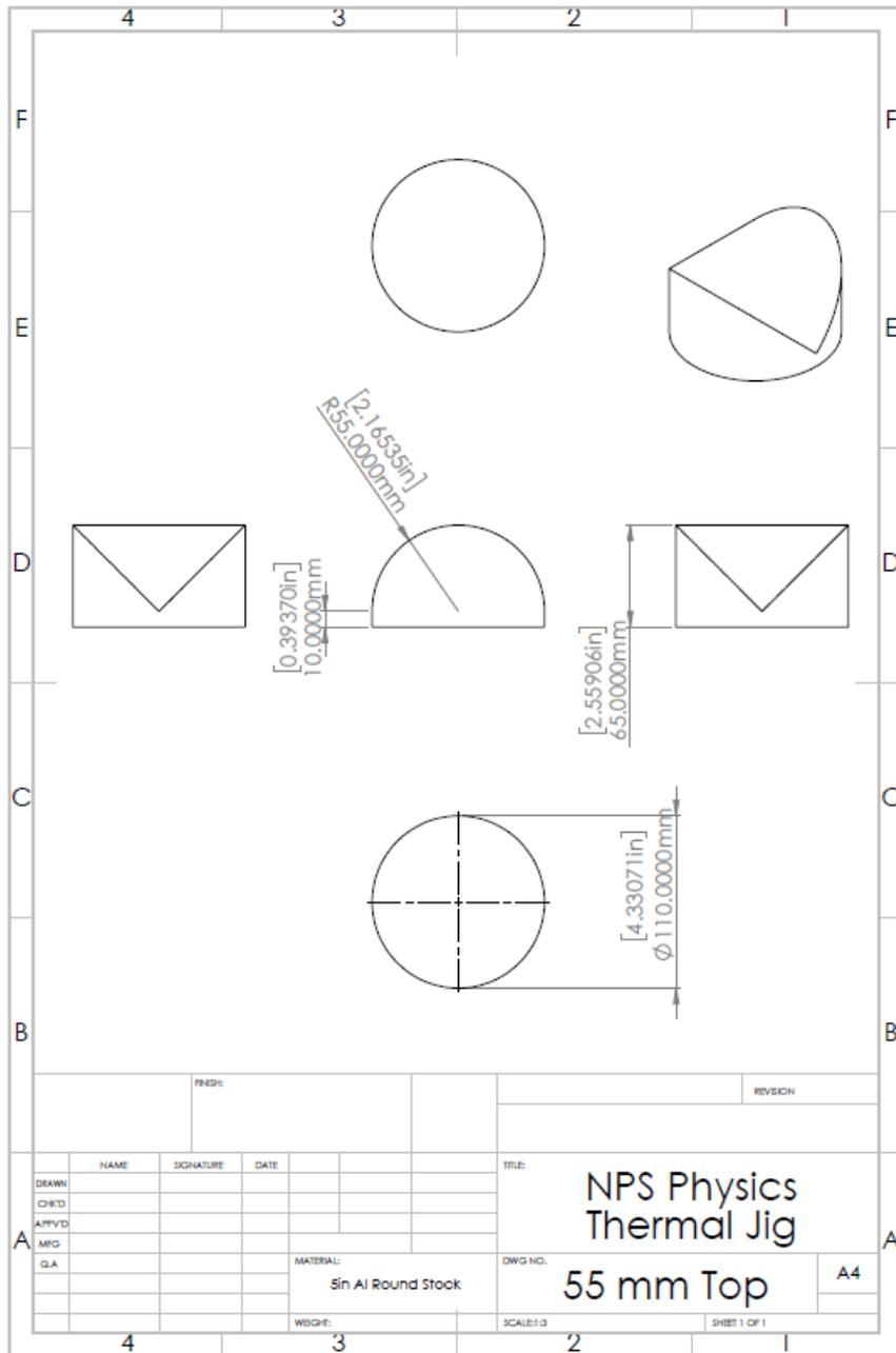
Figure C.2. Jig Top for Composite with  $r=50$  mm
