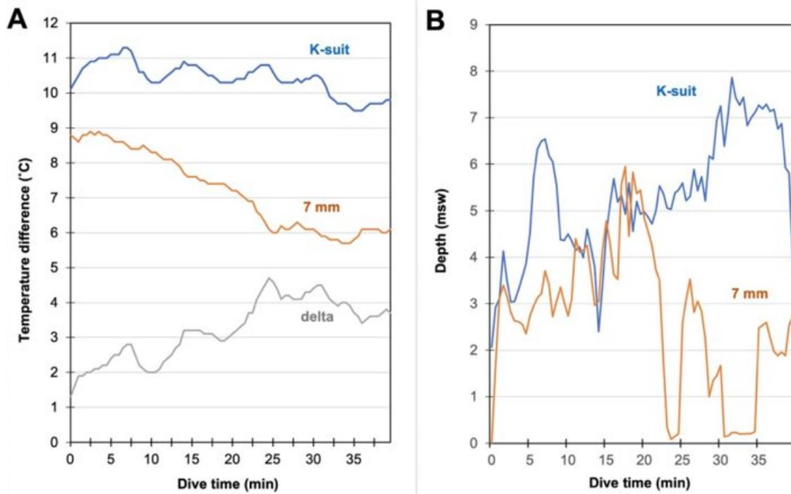
Figure 2.12. This field test supports the theory that incorporating stiff composites into a thinner neoprene wetsuits can produced comparable or superior  $\Delta T$  results Source: [18]
