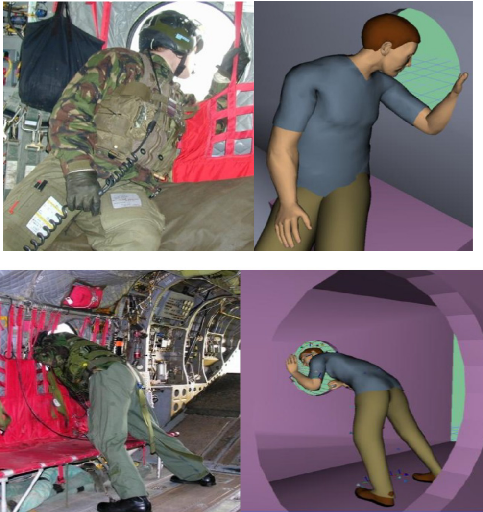
Figure 6-9: Actual and Digital Human Model Posture Recorded Using Motion Capture Data. Photos reprinted with permission from QinetiQ.
