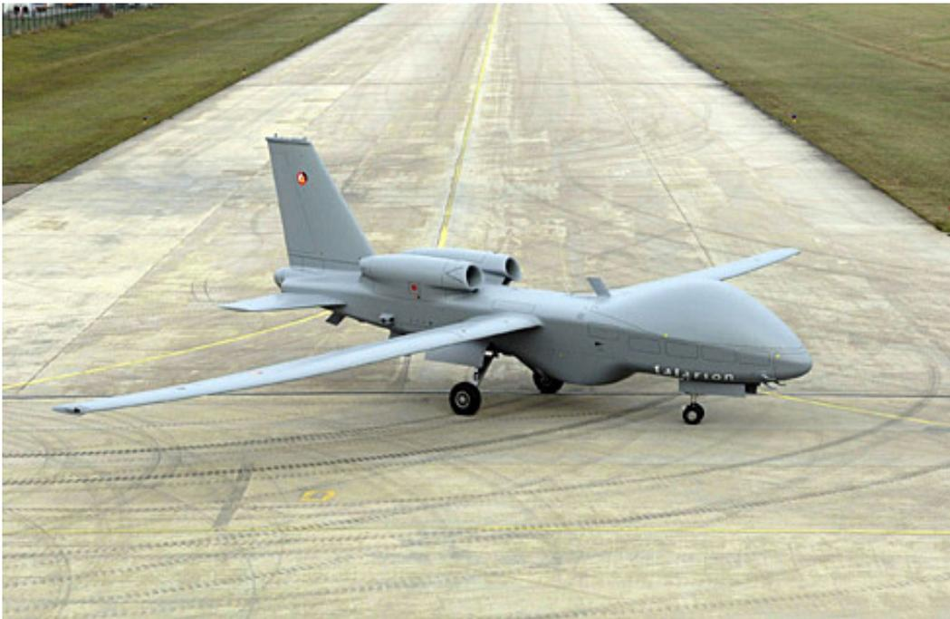
**Figure 14-2: MALE UAV Mock-Up (Airbus Talarion).**
