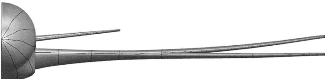
**Figure 6-7: Initial Fluid Mesh in 1 G Cruise Flight Conditions and Corresponding Jig Shape.**
