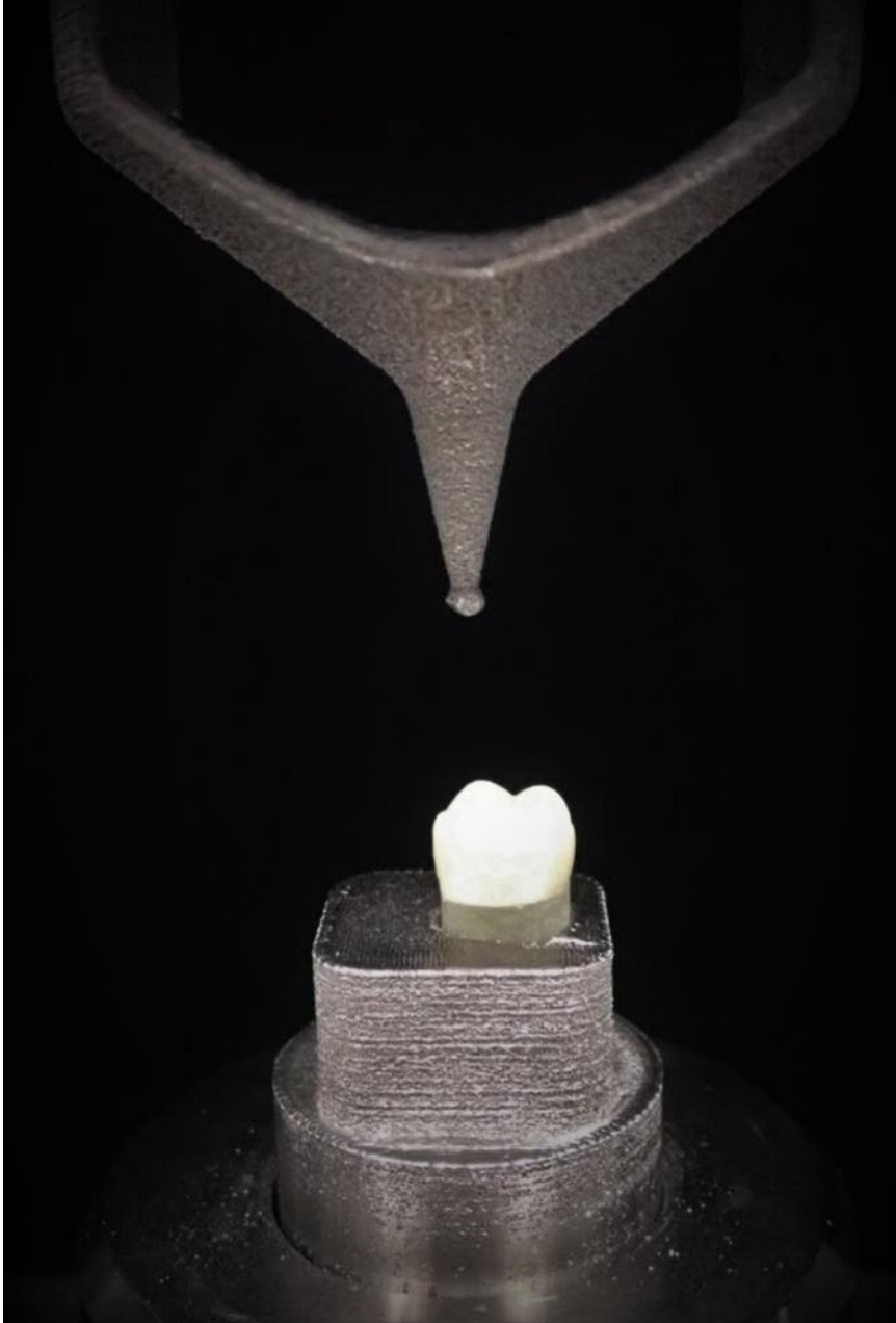
Figure 3. Mounting jig and setup for load testing
