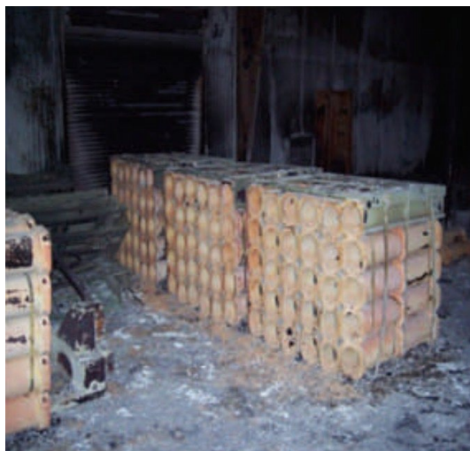
Figure 5 MACS charge after FCO test
