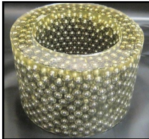
Figure 10 Melt liner for controlled fragmentation
