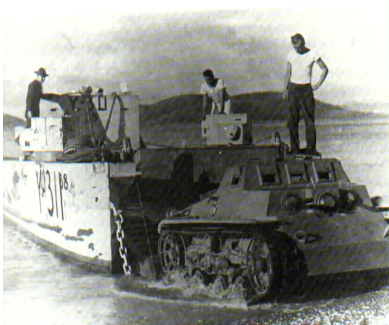
Figure 3. A Marmon Harrington Combat Tank Light (CTL) unloading from a 45-foot Tank Lighter
