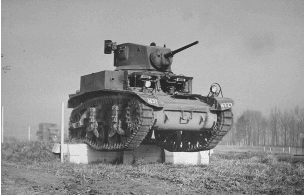
Figure 4. The M2A4 Light Tank in Pre-trials at Fort Knox
