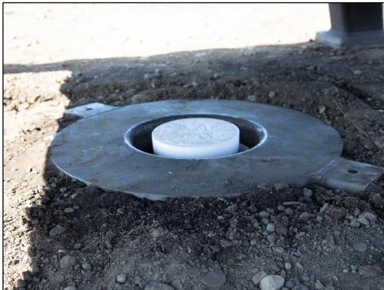
Figure 3: C4 explosive charge positioned in steel containment cylinder prior to a test event with top surface flush with top surface of steel containment cylinder.
