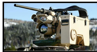
M153 Protector - CROWS II (Commonly Remotely Operated Weapon Station)
