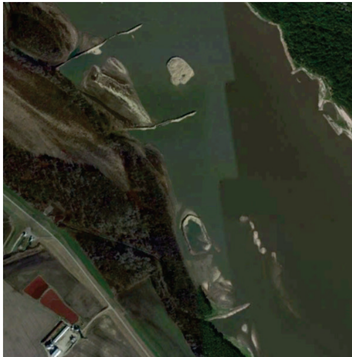
Figure 5. Filled chevron and downstream placement in visible in November 2013 Google Earth imagery. (from Google Earth Pro 2021)
