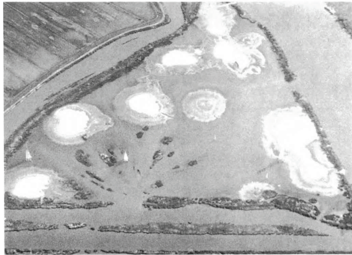
Figure 16. Aerial image of Donlon Island immediately after placement in 1985 to create nine dredged material islands (from England et al. 1990).
