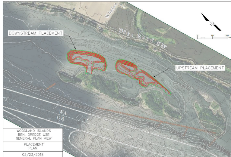
Figure 19. Planned terrain features (brown concentric lines) that were constructed using sediments dredged from the federal navigation channel. Only the downstream feature (see also Figure 21) was constructed due to the limited amount of dredged sediment available (from USACE Portland District 2020).
