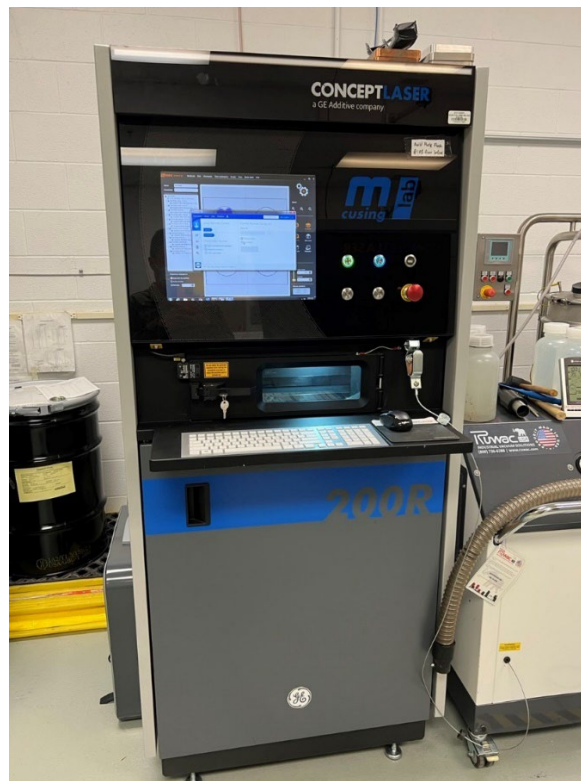
Figure 3. Concept Laser Mlab Cusing 200R 3D metal printer.
