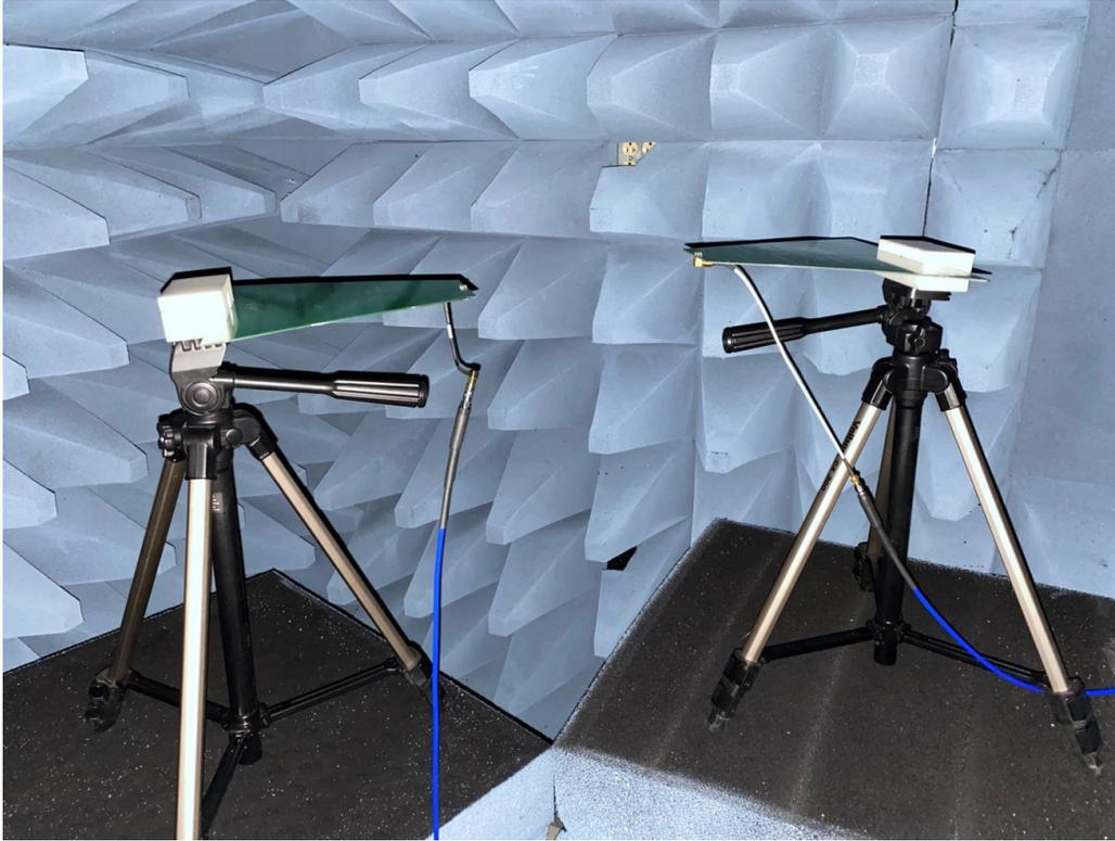
Figure 35: Free Space Loss and Test Antenna Calibration
