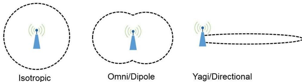
Figure 4: Antenna Propagation
