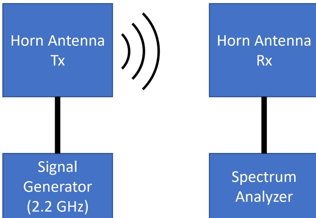
Figure 26: Experimental Setup 5
