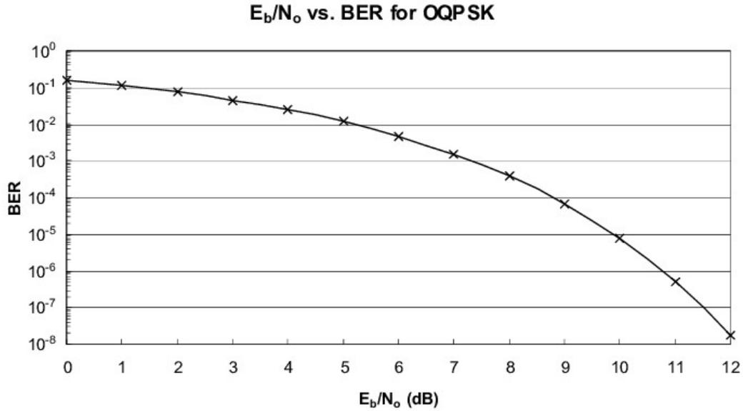
Figure 32: Bit Error Rate Probability of OQPSK Modulation [19]
