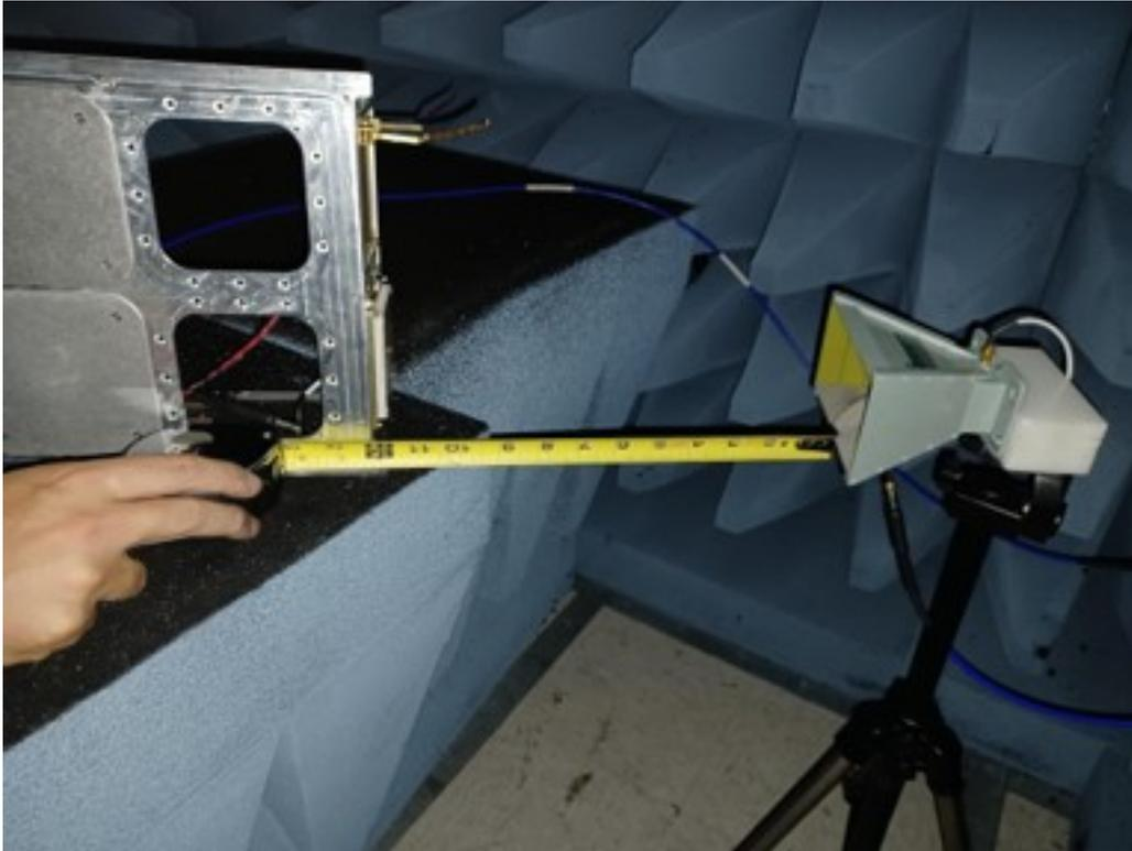
Figure 43: GM1 S-Band Patch Antenna Test Setup
