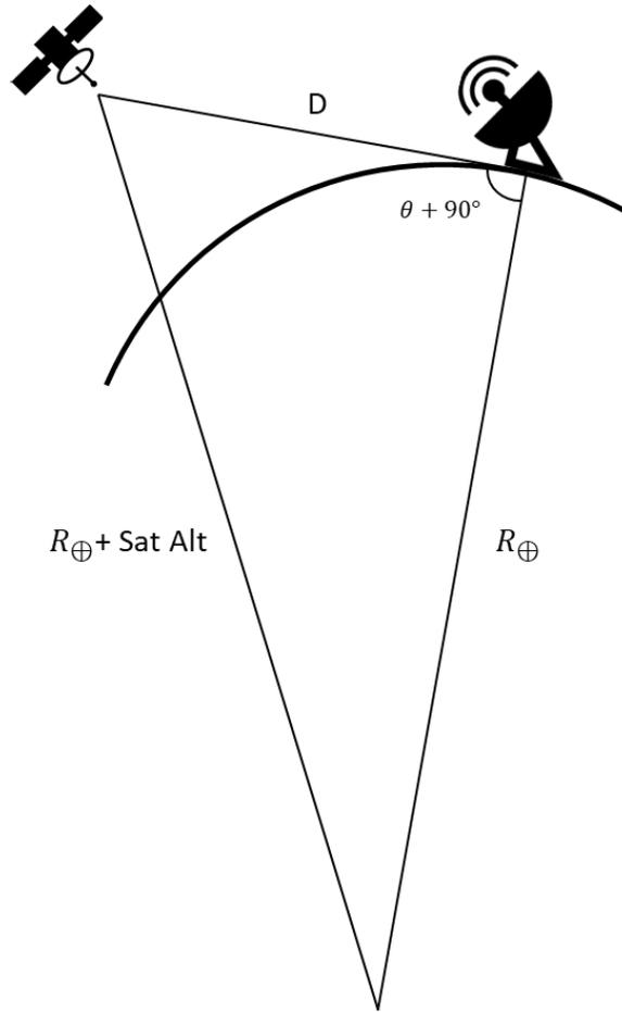
Figure 31: Radio Link Geometry
