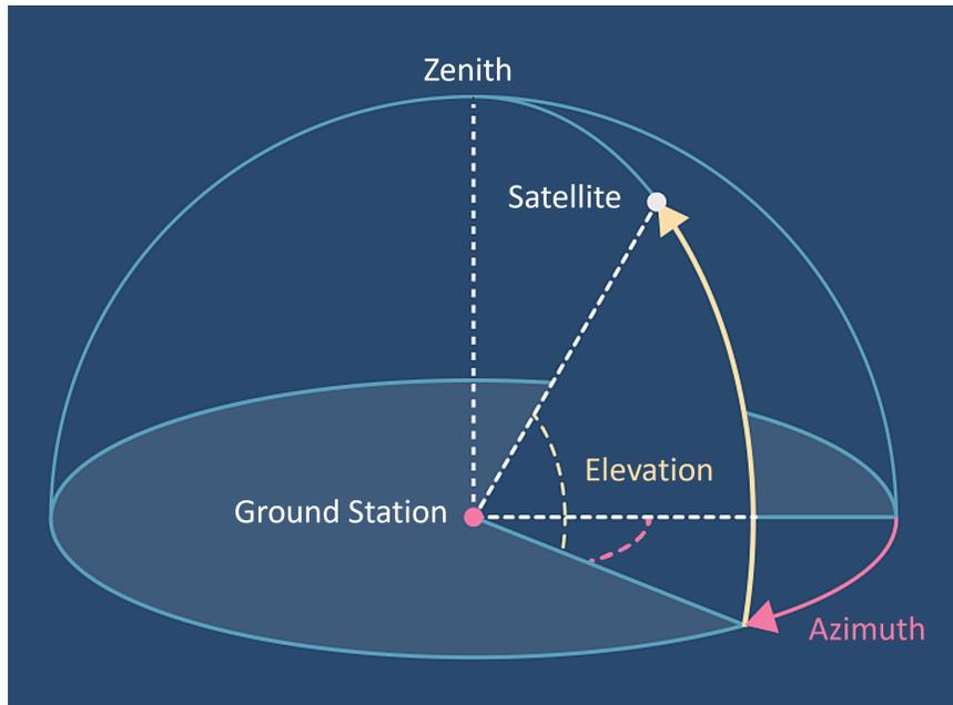
Figure 5: Illustration of Azimuth and Elevation angles
