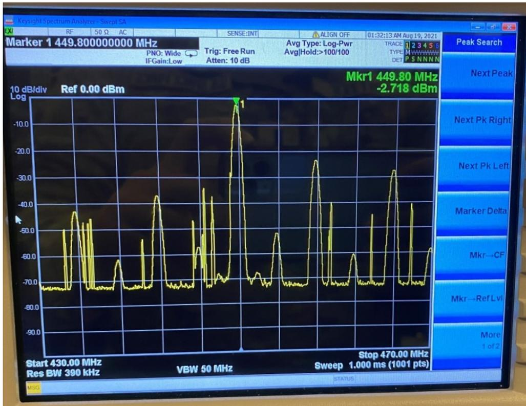
Figure 48: Cadet PLUS Uplink Test Measurement
