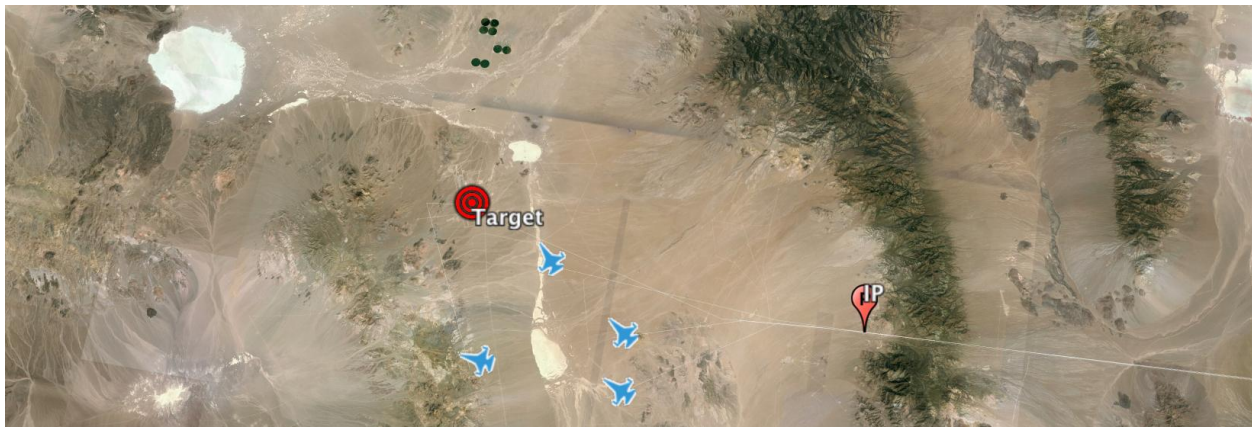
Figure 8. Map view of course deviations caused by GPS spoofing, as target is approached and missed.
