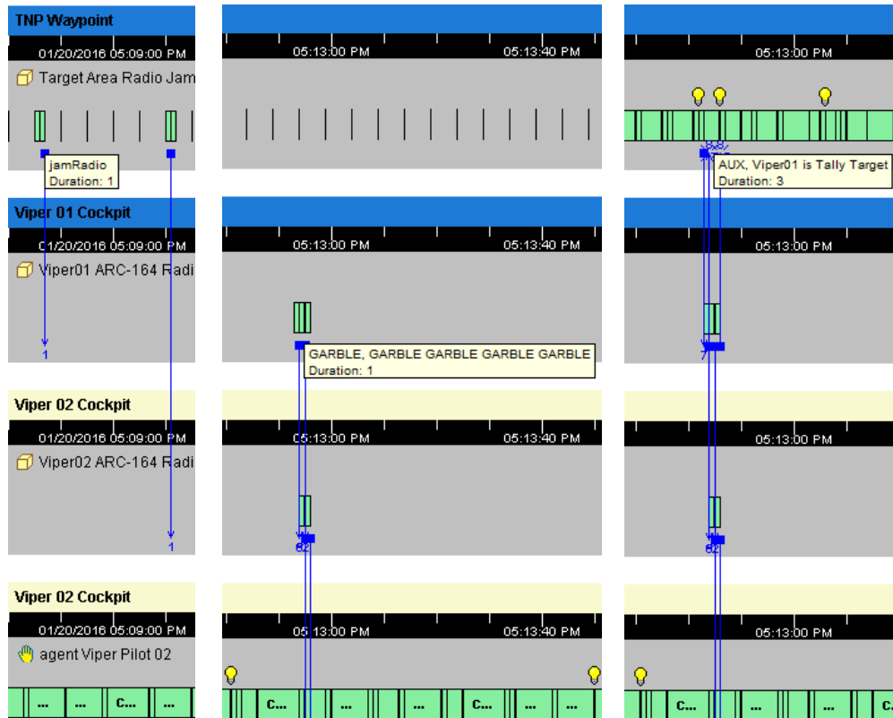
Figure 6. Jamming effects (left) result in garbled comms (center) and Viper 02 failing to locate target (right).
