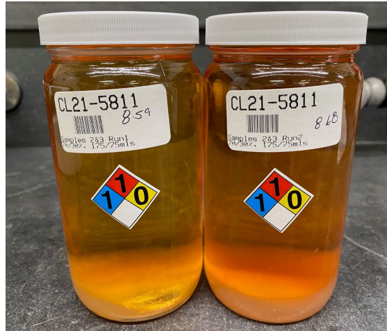
Figure 11. White Precipitates Formed Post- ASTM D4340 on ELC Blends
