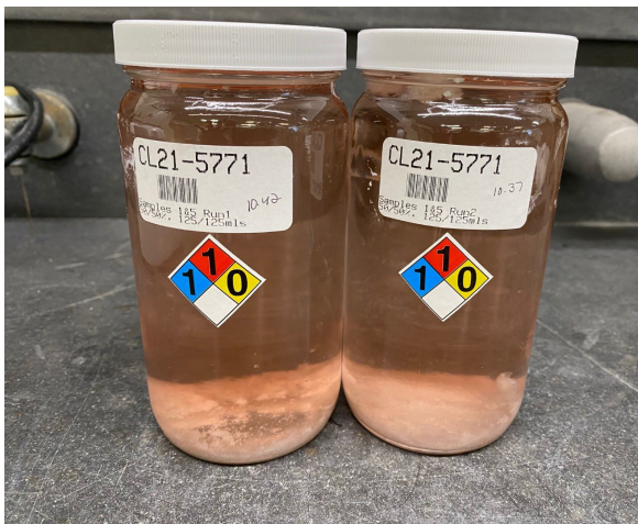
Figure 11. White Precipitates Formed Post- ASTM D4340 on ELC Blends
