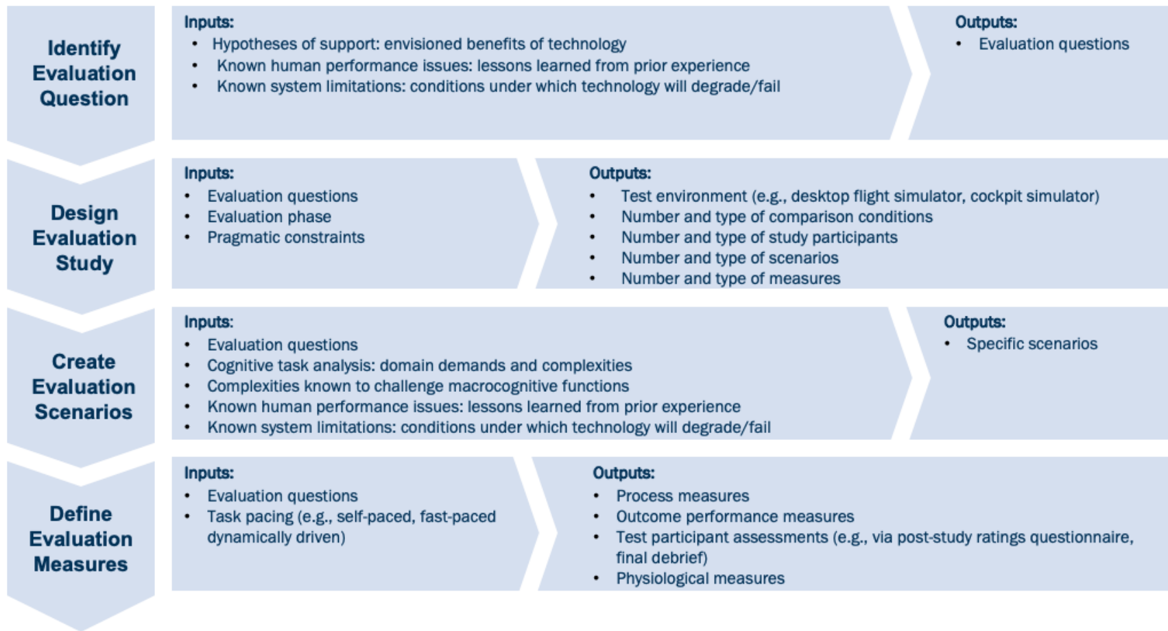
Figure 4 Considerations that go into design of an evaluation study and selection of evaluation measures
