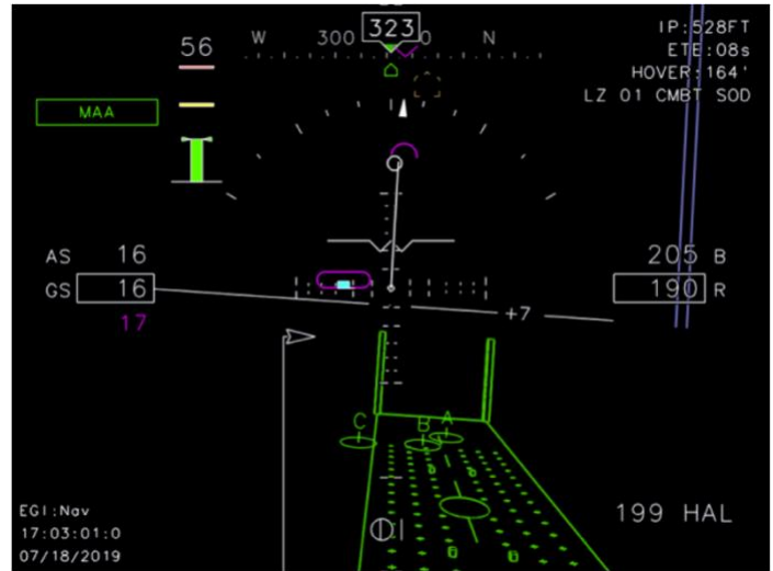
Figure 3 from Szoboszlay et al. (2021) depicting artificial landing pad symbology with options A, B, and C as identified by the safe landing area determination algorithm.
