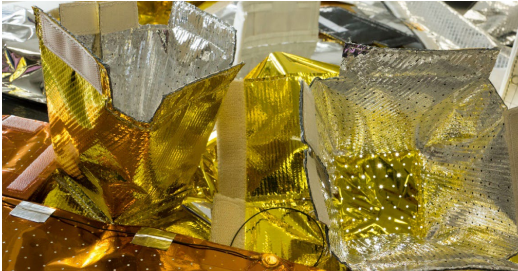
Fig. 5.1 Example of Multilayer Insulation [24]
