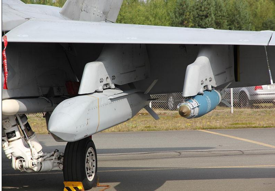
Figure 13. AGM-158 Attached to an F/A-18D Hornet
