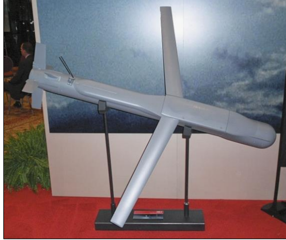
Figure 10. Model of a GBU-53 Small Diameter Bomb II
