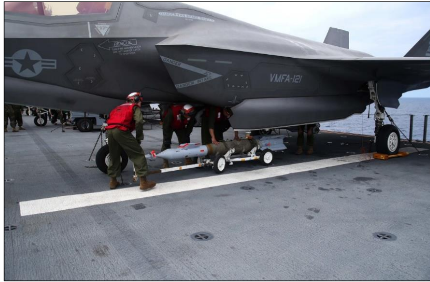
Figure 6. Loading a Paveway II into an F-35B
