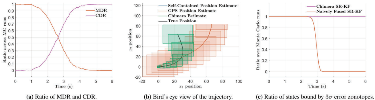
Figure 6. Monte Carlo validation of the Chimera SR-KF estimator and detector during spoofed conditions for the linear, double-integrator system
