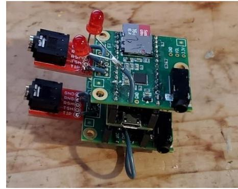
**Figure 17 - The Teensy datalogger**
