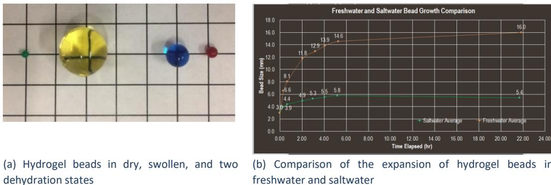
Figure 6. Illustration of the expansion of the hydrogel beads under different conditions
