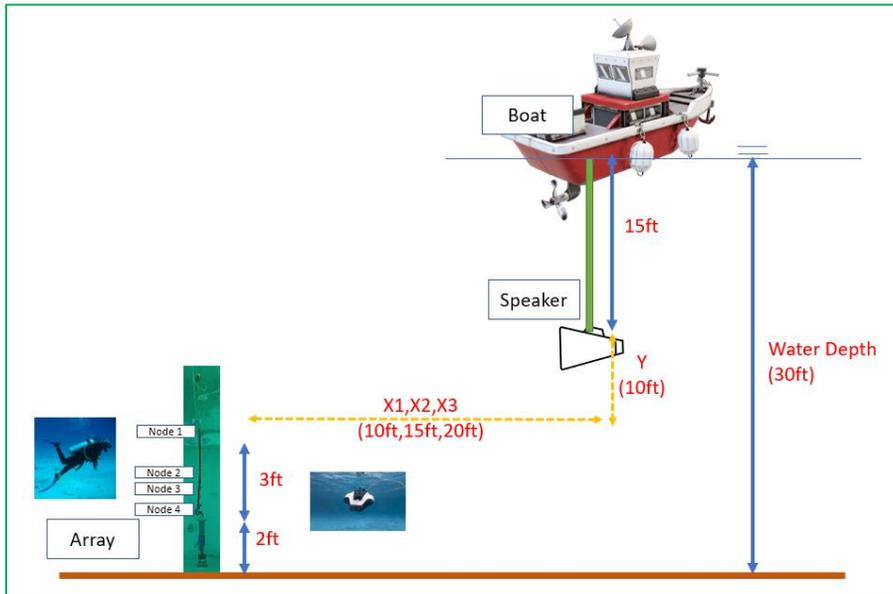
**Figure 27. Lake Denton test setup.**
