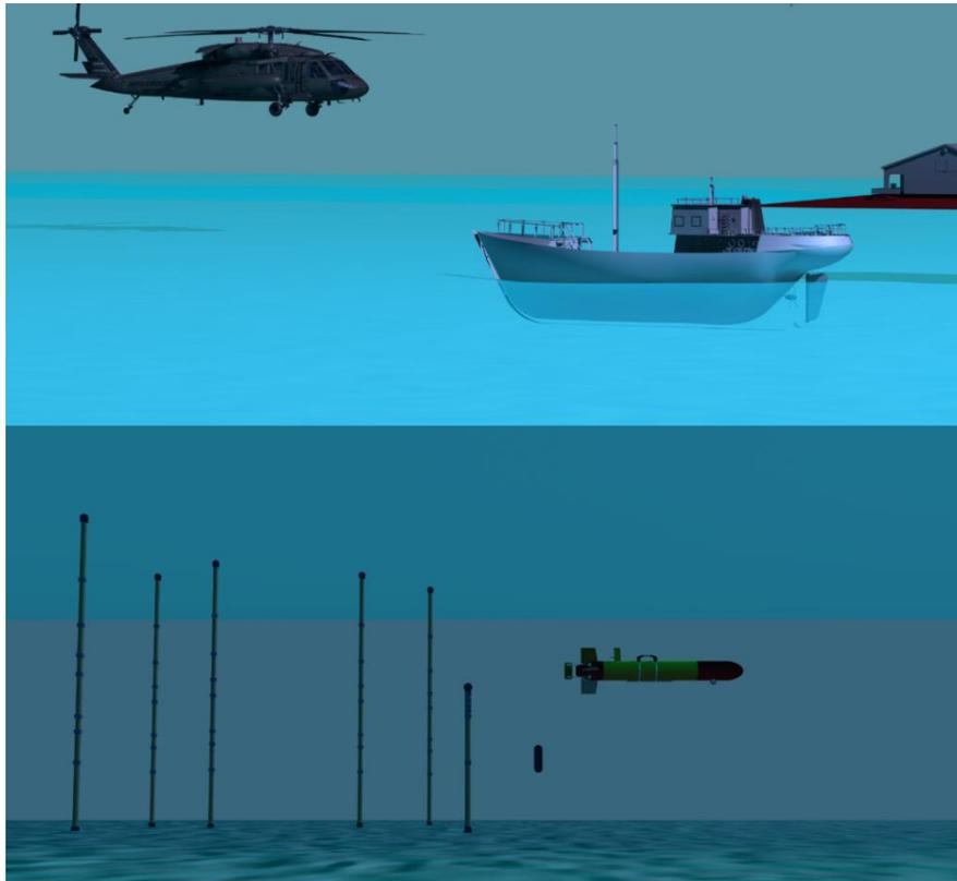
**Figure 1. The illustration of UDSN consists of multiple UICSA nodes that can be deployed from aerial planes, boats, or AUVs.**
