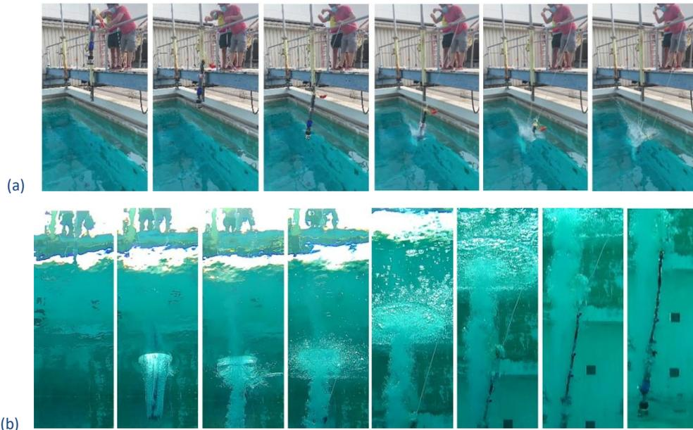
**Figure 23. Deployment of the 7-element array. (a) Video frames capture the release process above water. (b) Video frames capture the underwater portion of the release process.**
