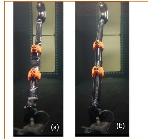
**Figure 12. 4-element HBE based UICSA expansion process**
