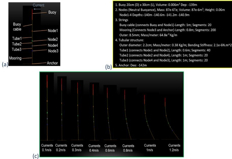
Figure 5. Illustration of the Simulation of a 4-node UICSA structure using OrcaFlex
