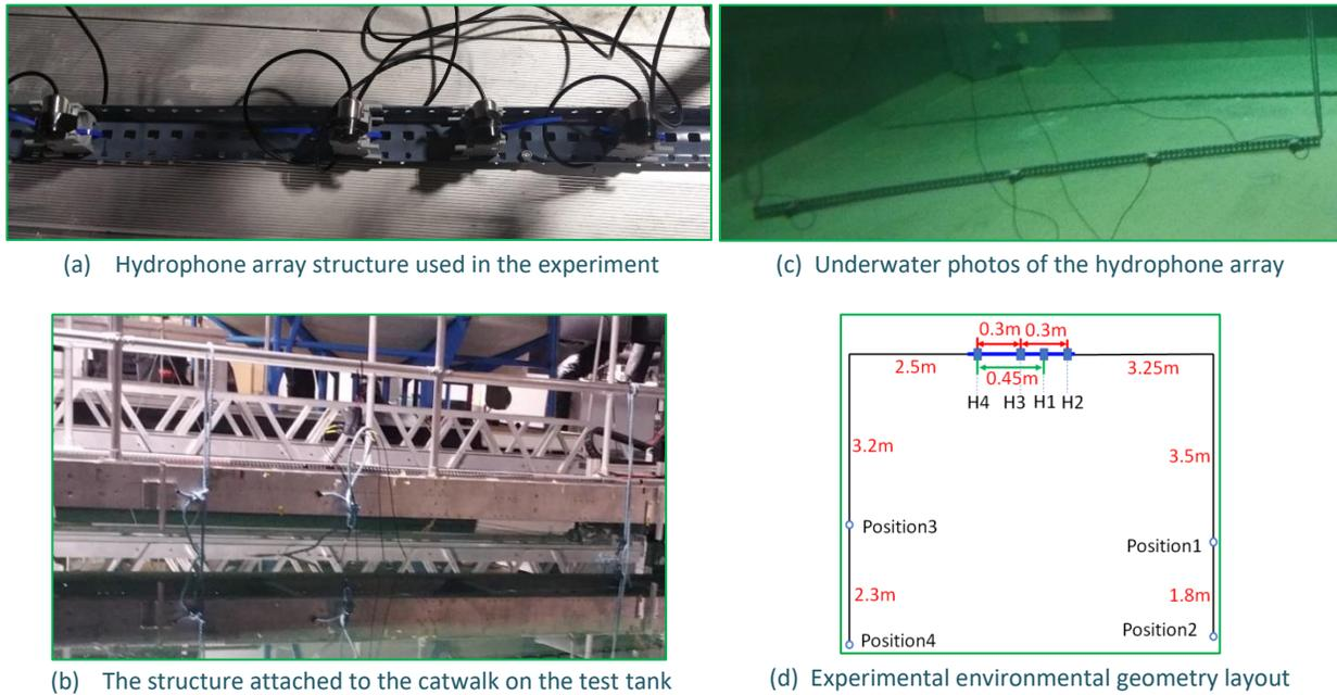
**Figure 2. Experimental layout and environment.**
