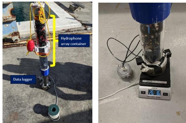
**Figure 22. Aquagel based 7-element UICSA array**
