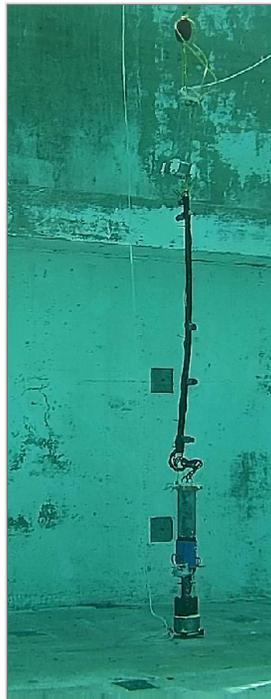
**Figure 24. The array status ten minutes after the release. The array can be seen to be fully expanded.**
