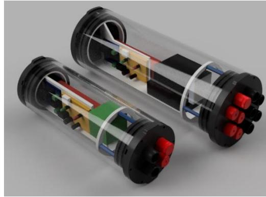
**Figure 19 - Completed housings for the Teensy and BEAST**
