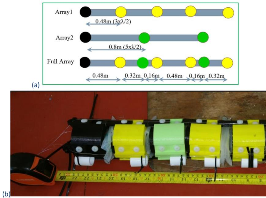
**Figure 3. 7-node UICSA sensor configuration. (a) Illustration of the array geometry (b) The actual prototype**
