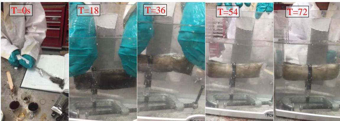
**Figure 7. Time lapsed sequence (at 18-second intervals) to illustrate the expansion of HF402 foam**
