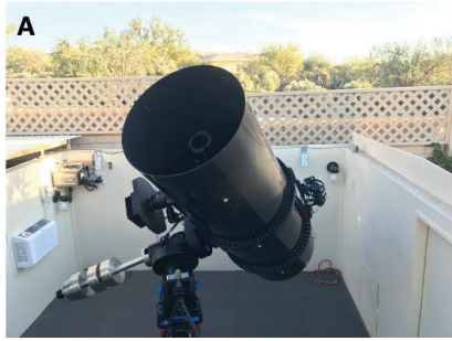
Location: Tucson, Arizona, USA Aperture: 0.5-meter Focal Ratio: F/2.8 Field of View: 1.4 x 1.4 deg Pixel Scale (1x bin): 1.22"/pixel Focus: Multi-color photometry
