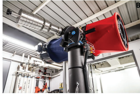
Location: Tucson, Arizona, USA Aperture: 0.6-meter Focal Ratio: F/4 Field of View: 16 x 16 arc min Pixel Scale (1x bin): 0.93"/pixel Focus: Visible Spectroscopy
