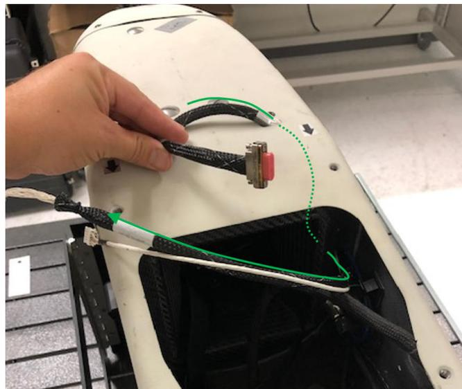
Figure E-17. MAIM-Payload Cable Run
