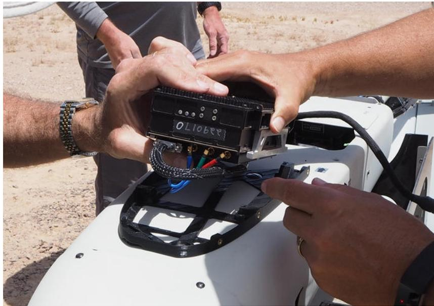
Figure E-8. Stalker Primary Mount – Payload Installation (1 of 3)
