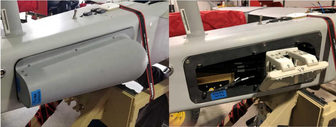
Figure D-16. Jump-20 Side Hatch Antenna Mount – With Radome (left), Without Radome (right)
