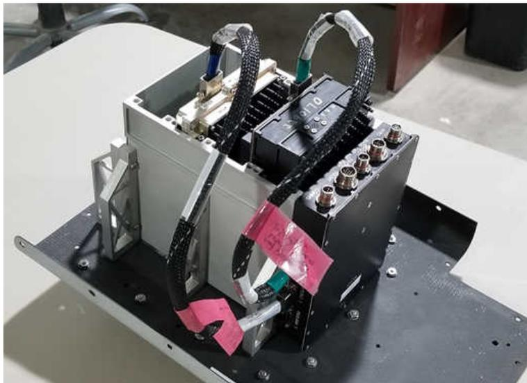
Figure D-20. MAIM-Payload Cable Runs
