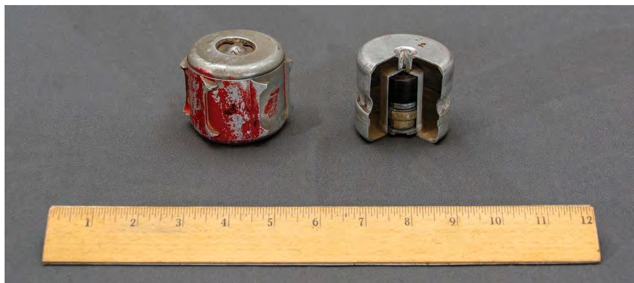
Figure 43: Bomblet, 2.5-inches, E139 - Photograph - Right: Exterior; Left: Cutaway View
