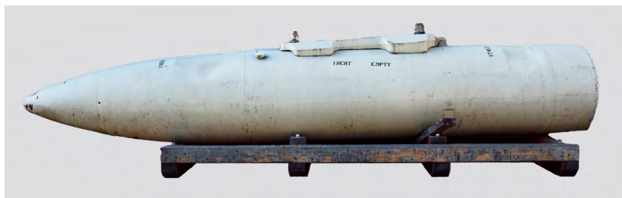
Figure 166: Tank, Aircraft, TMU-28/B - Photograph
