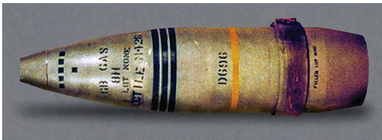
Figure 219: Projectile, 8-inch, Howitzer, M426 – Photograph
