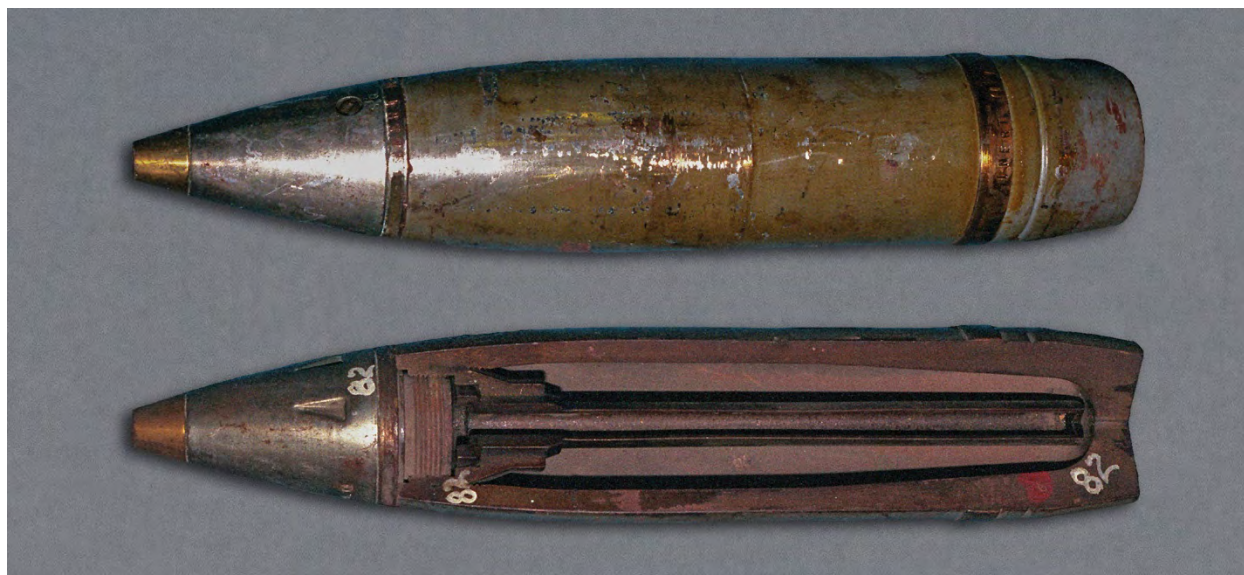
Figure 185: Projectile, 75-mm, M64 – Photograph - Top: Intact, Bottom: Cutaway View
