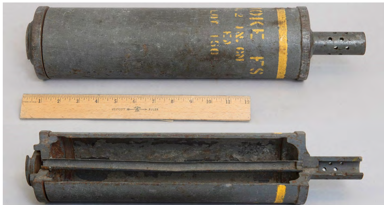
Figure 175: Mortar, 4-inch, MI, Stokes - Photograph - Top: Exterior View, Bottom: Cutaway
