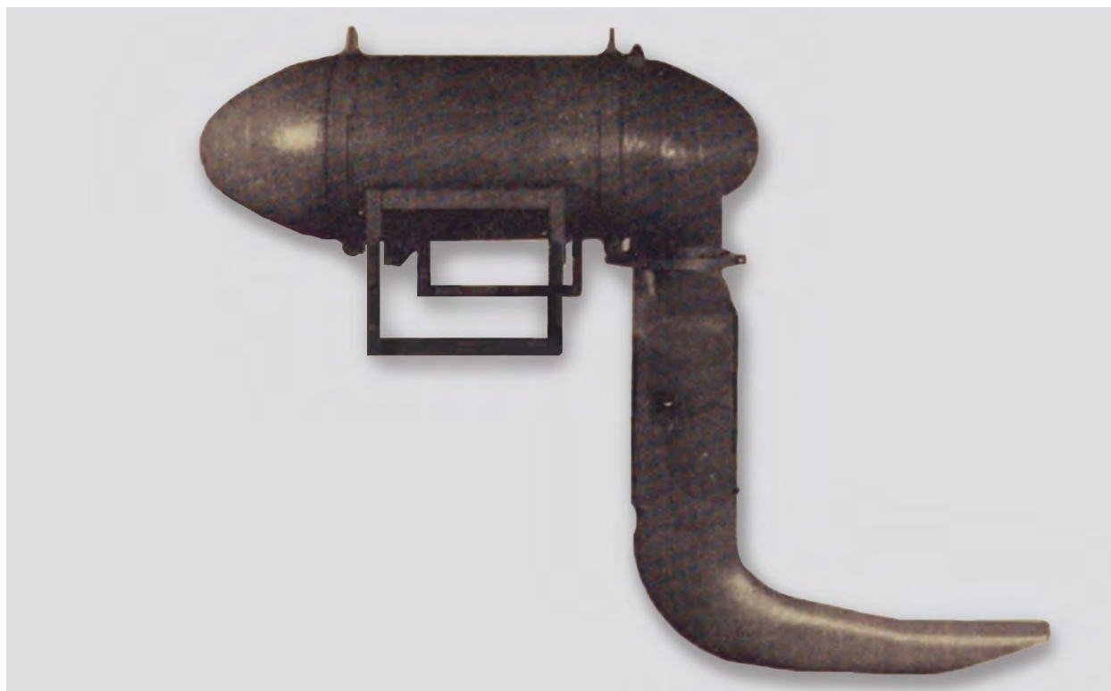
Figure 161: Tank, 70-gallon, Airplane, M33 and AN-M33A1 – Photograph
