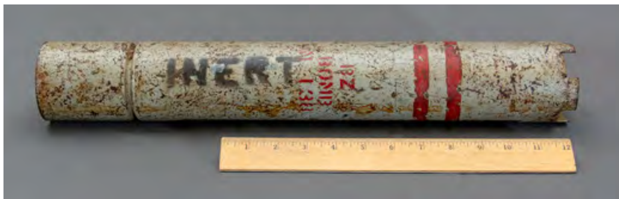
Figure 78: Bomblet, 10-pound, M138 – Photograph
