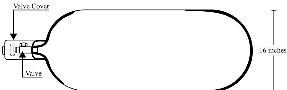
Figure 143: Cylinder, 300-pound – Line Drawing
