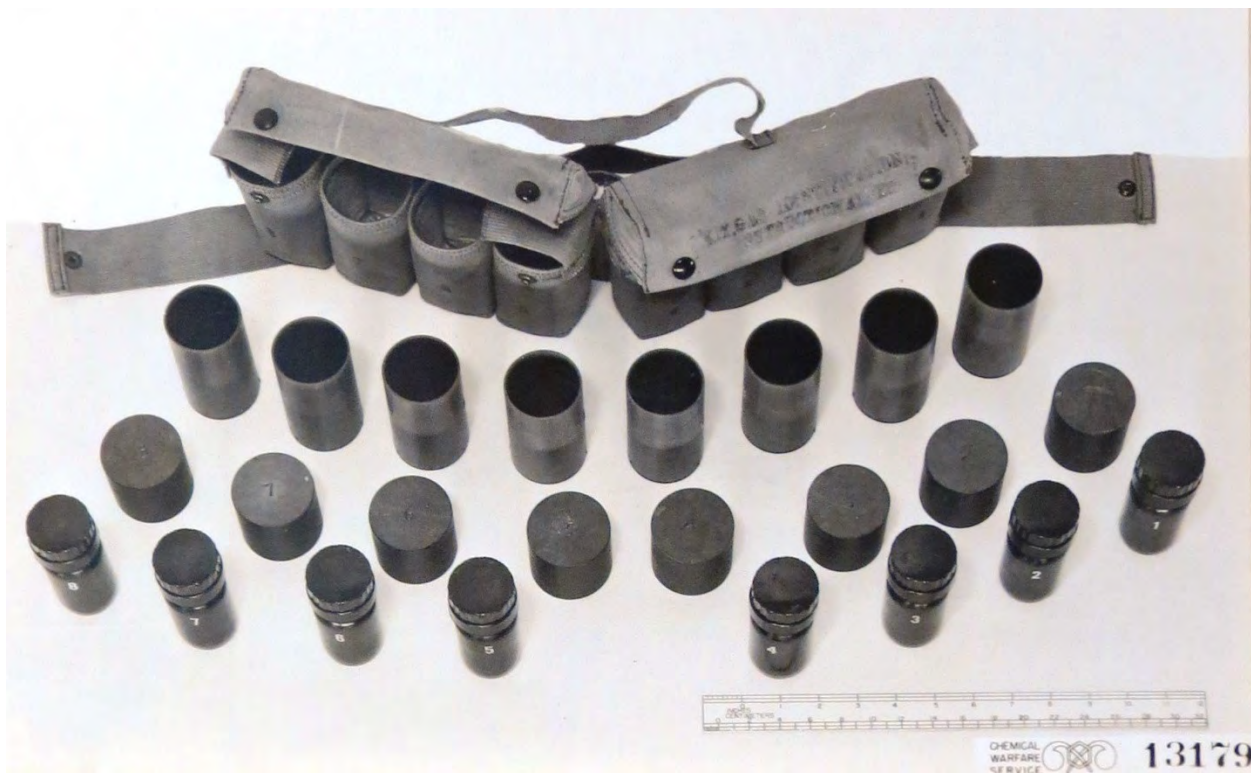
Figure 99: CAIS, Gas Identification Set, Instructional, M2 - Photograph
