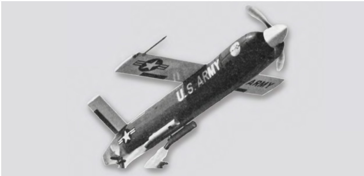
Figure 145: Drone Weapon System, Multipurpose, AN-USD-2 - Photograph
