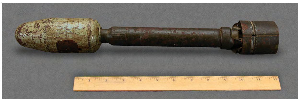
Figure 230: Rocket, 2.36-inch, M10 - Photograph
