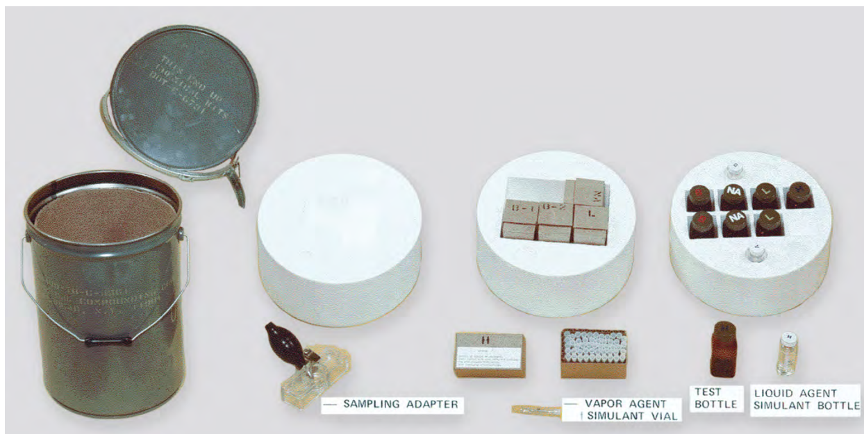
Figure 108: SCAITS, M72A2 - Photograph
