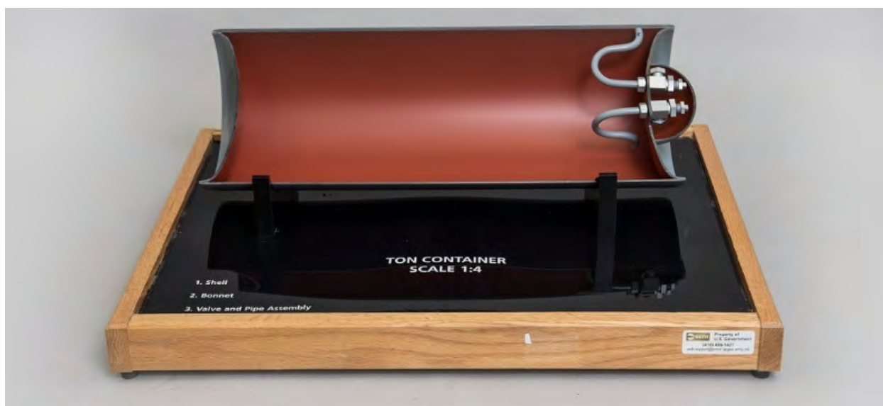
Figure 134: Container, Bulk, One-ton, Type A - Photograph – Container Replica, Cutaway View
