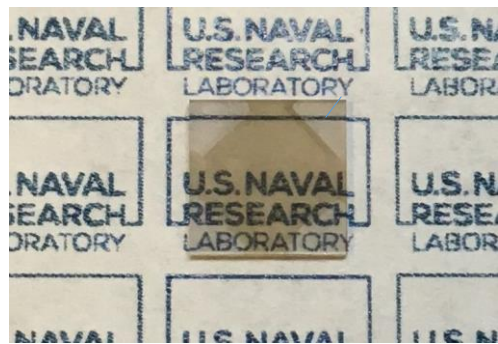
Fig. 6: Optical image of BN film grown on 6x6 mm 2 diamond IIa (100) CVD substrate. H-BN and c-BN are distinguished by color. H-BN films are grey color as shown in the image, while c-BN films are colorless and undistinguished from diamond substrate. Corner features are footprint of MBE sample holder.
