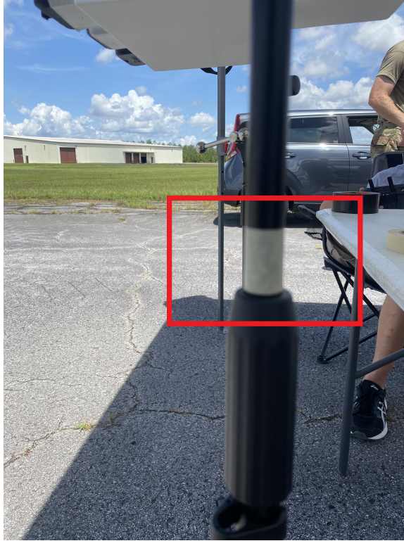
Figure 32: Tape Used To Set 1 m Height
