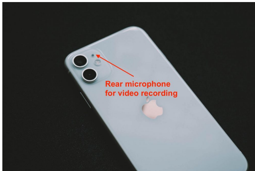
Figure 23: Rear MEMS Microphone Location [38]
