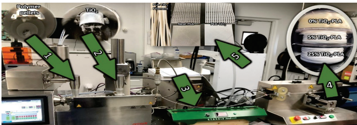
Figure 5. Compounding of photocatalytic \text{TiO}_2 into the 3D printable polymer polylactic acid (PLA). Step 1: pure polymer pellets fed into the extruder; step 2: pellets melted and compounded with \text{TiO}_2 ; step 3: composite filament is cooled; step 4: filament is spooled; step 5: \text{TiO}_2 polymer composite filament is 3D printed into structures for HAB treatment efficacy testing. Photographs by A. Kennedy.
