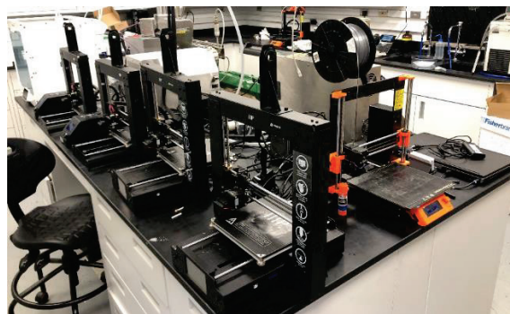
Figure 4. An additive manufacturing laboratory at ERDC-EL including fused filament fabrication printers and extruders. Photo by Alan Kennedy.
