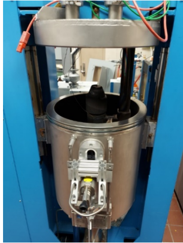
Figure 30: Loading the die and punch assembly into the enclosure for SPS.
