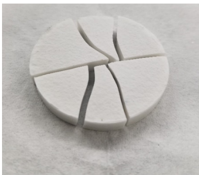
Figure 35: A damaged 40-mm diameter LuAG puck following processing with several distinct cracks through the thickness.
