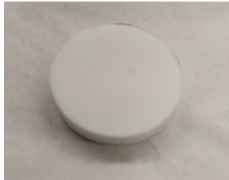
Figure 34: 40-mm diameter LuAG puck following sintering and heat treatment.
