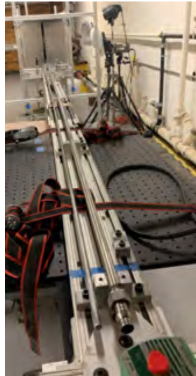
Figure 14: Stainless Steel Gas Gun Barrel 12 feet Long with a 0.525 inch inner diameter
