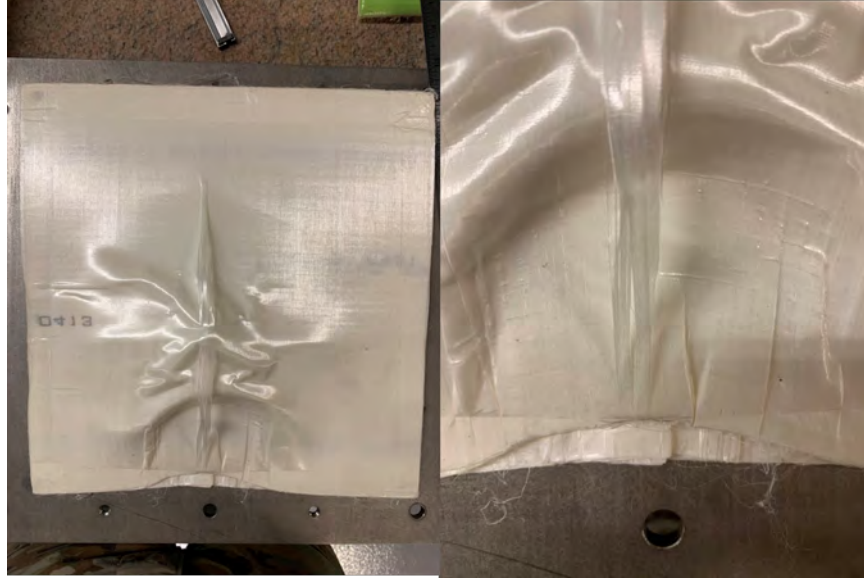
Figure 31: Inter-laminar Shear on Plate 2 of UHMWPE
