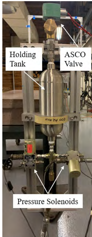
Figure 13: Pressure Holding Tank with Pressurization Solenoids and Firing Valve
