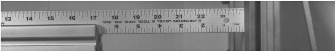
Figure 23: Camera Calibration Image Showing the Camera Field of Vision and the Ruler Scaled by Inches Used to Set the ft/pixel Calibration
