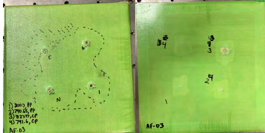
Figure 40: Kevlar ® KM2, 600 Denier Plate Following 4 Shot Grid, Left: Front View, Delamination Outline Marked, Right: Rear View, Note Visible Delamination Around the Point of Impact as Well as the Discoloration where the Plate was Clamped.
